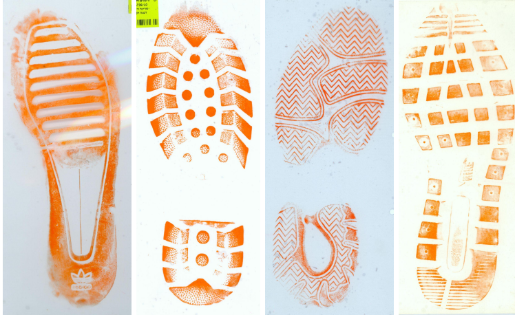
Figure A.6: Examples from an existing shoeprint dataset [102]. We use these prints as a starting point for synthetic depth map generation. Note that even though these are shoeprints collected under a controlled lab environment, the images are still quite noisy. This necessitates some preprocessing before these can be used for synthetic depth map generation.
