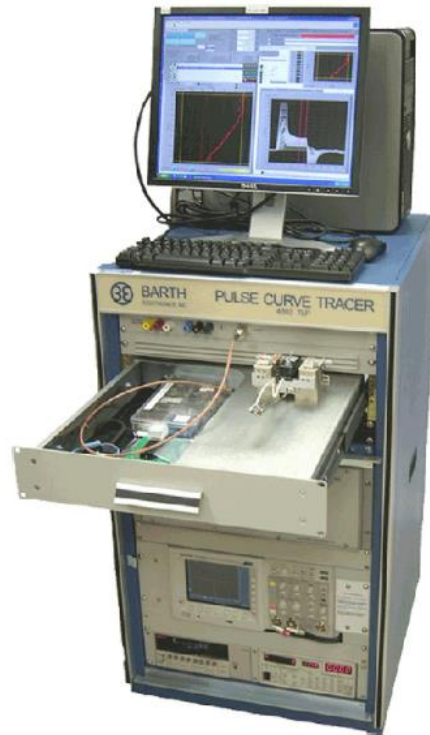
Fig. 2.13 BARTH Model 4002 TLP tester used for TLP testing.
