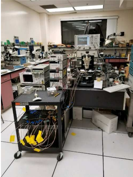
Figure 5.2: Four port network analyzer, probe station with microscope, broadband bias tees, and hybrid coupler network used to test the SSDL circulator.
