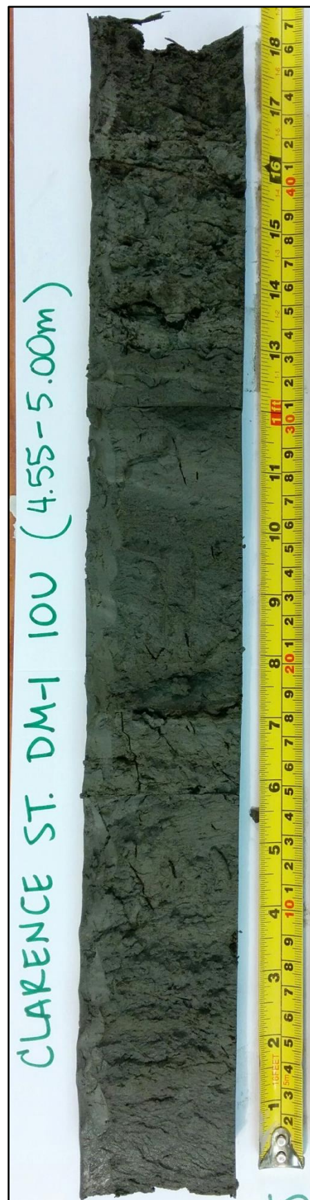
Figure B.1-38: S37-DM1-10U (4.55-5.00 m BGS)
