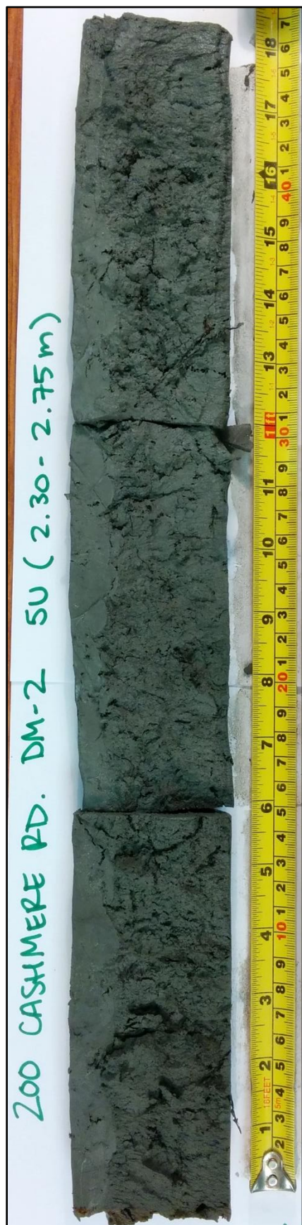
Figure B.1-19: S33-DM2-5U (2.30-2.75 m BGS)
