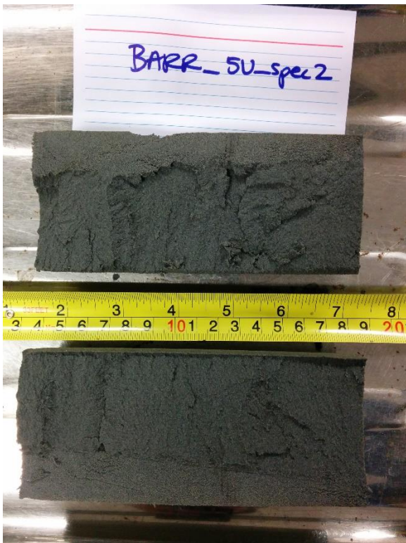
Figure C.3.2-8: S14-DM2-5U-B, Tested (mechanical issue during testing – CTX data not used)
