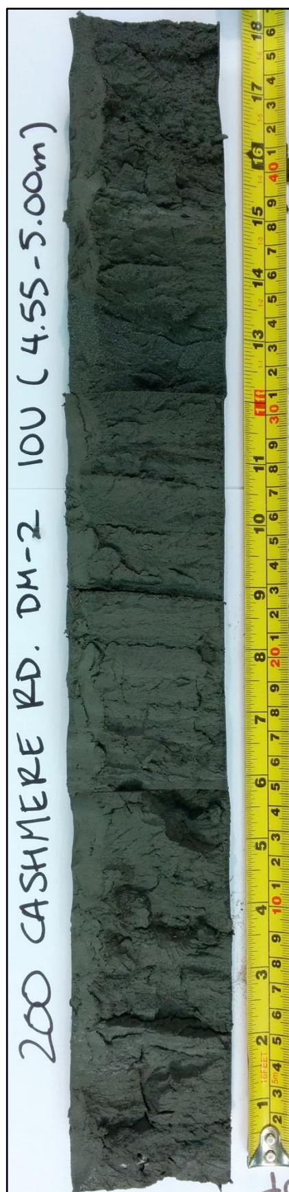
Figure B.1-24: S33-DM2-10U (4.55-5.00 m BGS)
