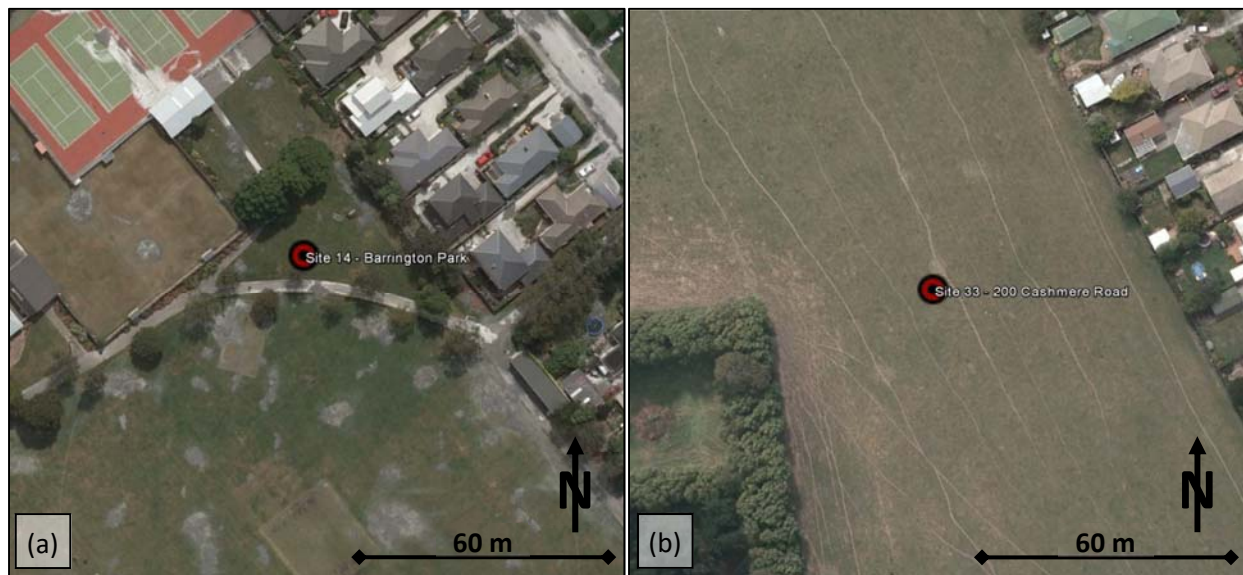
Figure 2.8: Aerial photographs at: (a) Site 14 (liquefaction observed) and (b) Site 33 (no liquefaction observed) after the 22 FEB 2011 Christchurch earthquake. The light brown marks in (b) are stock tracks from livestock. (modified from NZGD and Google Earth™).
