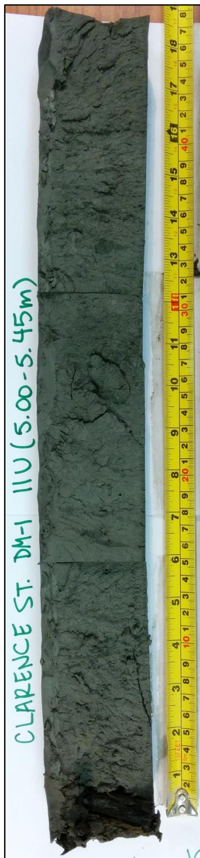
Figure B.1-39: S37-DM1-11U (5.00-5.45 m BGS)
