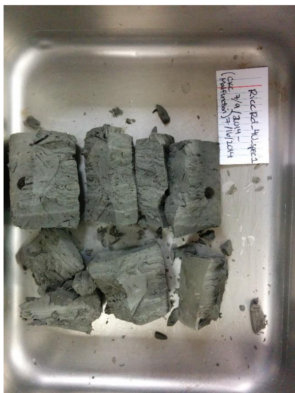
Figure C.3.4-6: S23-DM1-4U-A, After Testing Attempted (CKC equipment malfunction)
