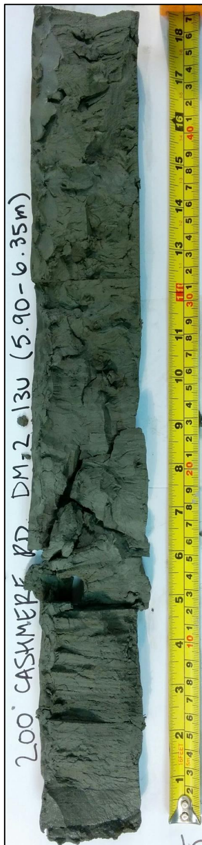
Figure B.1-27: S33-DM2-13U (5.90-6.35 m BGS)
