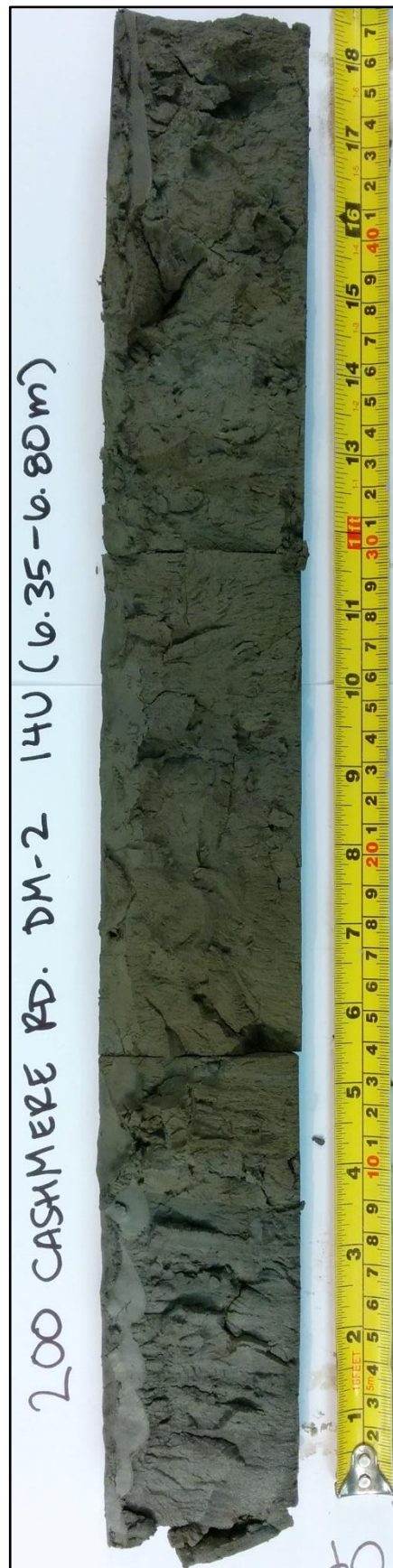
Figure B.1-28: S33-DM2-14U (6.35-6.80 m BGS)
