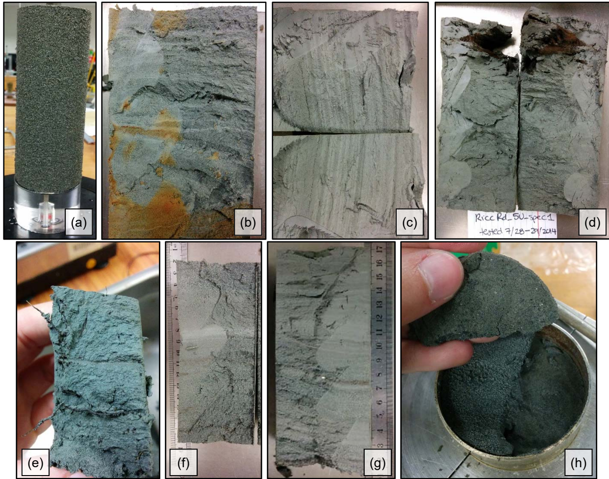
Figure 4.5: Representative CTX test specimens demonstrating varying degrees of heterogeneity. Acceptable: (a) Clean Sand (EQC3-DM1-5U-A), (b) PI=0 Silt (S21-DM1-3U-A), (c) PI=10 Silt (S33-DM1-8U-A), (d) PI=6 Silt (S23-DM1-5U-A), (e) PI=6 Silt (S23-DM1-7U-A). Acceptable, results require more interpretation: (f) Non-plastic Silty Sand/Silt (S33-DM1-6U-B), (g) PI=0 Silt (S33-DM1-7U-A). Unacceptable: (h) Clean Sand (S33-DM1-4U-B) – separation/void evident in tube, possibly disturbed during sampling.
