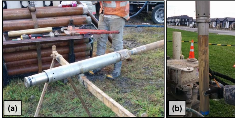
Figure 3.5: Dames & Moore hydraulic fixed-piston thin-walled sampler: (a) attached to drill rods (sample tube not attached), (b): with sample tube attached (immediately following sample removal from boring).
