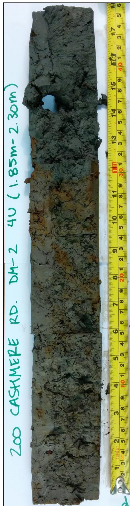
Figure B.1-18: S33-DM2-4U (1.85-2.30 m BGS) – void at ~ 37 cm is from large piece of wood in other half of sample
