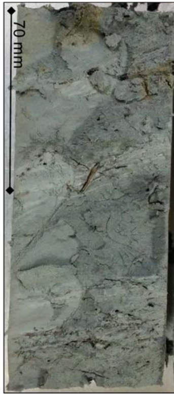
Figure 2.14: High-quality specimen (post-cyclic testing) from Site 23 (depth 3.39 m) showing layering from the stratified part of the CPT profile (specimen height approximately 14 cm). Note varying silt and sand content throughout specimen, silt laminations, and organic laminations/content.
