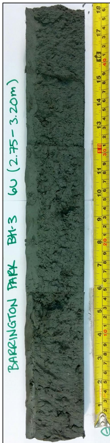
Figure B.1-6: S14-BH3-6U (2.75-3.20 m BGS)
