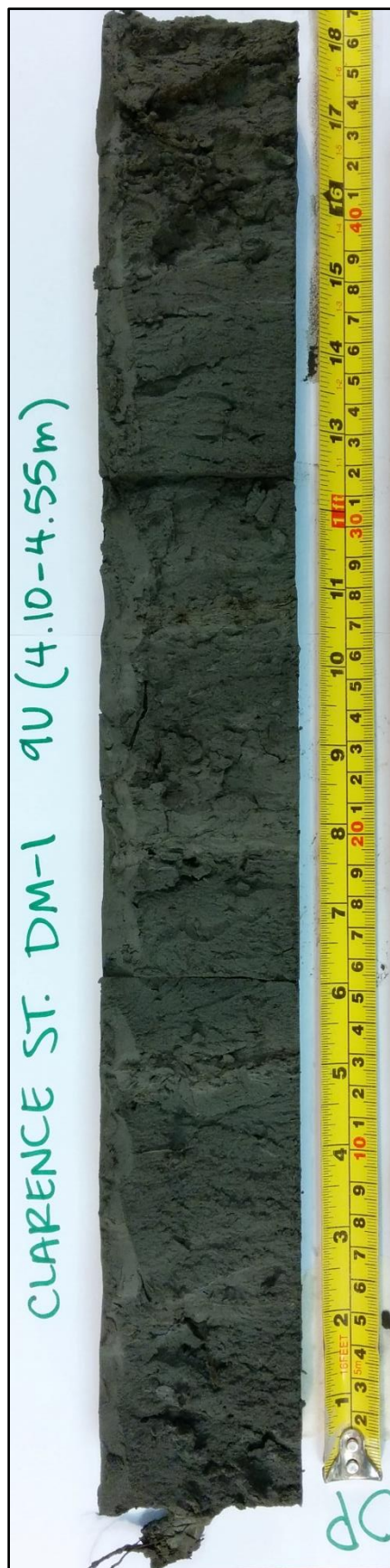
Figure B.1-37: S37-DM1-9U (4.10-4.55 m BGS)
