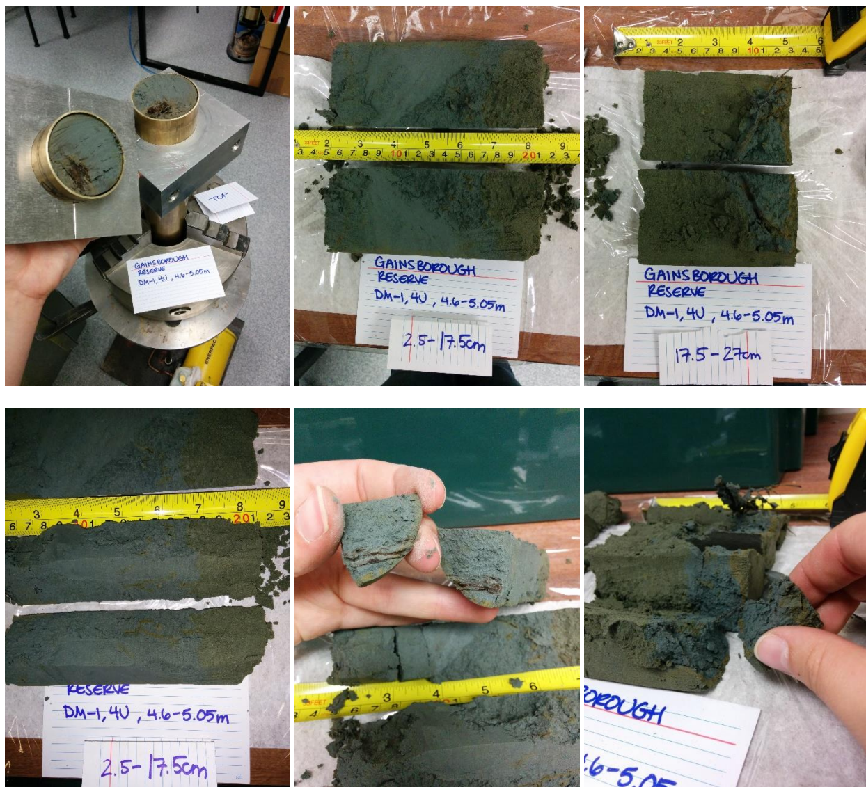
Figure C.3.1-5: S2-DM1-4U (not tested), As-Extruded
