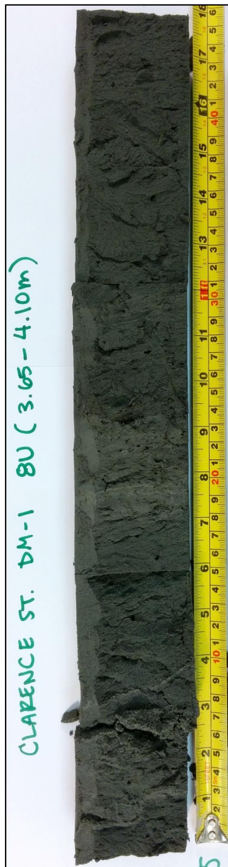
Figure B.1-36: S37-DM1-8U (3.65-4.10 m BGS)
