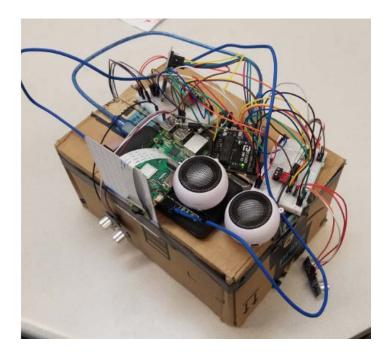
Third Eye is a system that assists people with impaired vision by using obstacle detection, facial detection and sound cues. The Third Eye prototype is embedded in a box representing a mock human.
