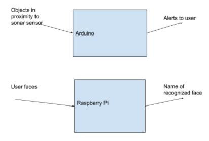
The components connected to the Arduino is one subsystem. The output of the Arduino are the alerts to the user. The input of the Arduino are potential obstacles in the environment. The components connected to the Raspberry Pi is another subsystem. The input of the Raspberry Pi are potential human faces.
