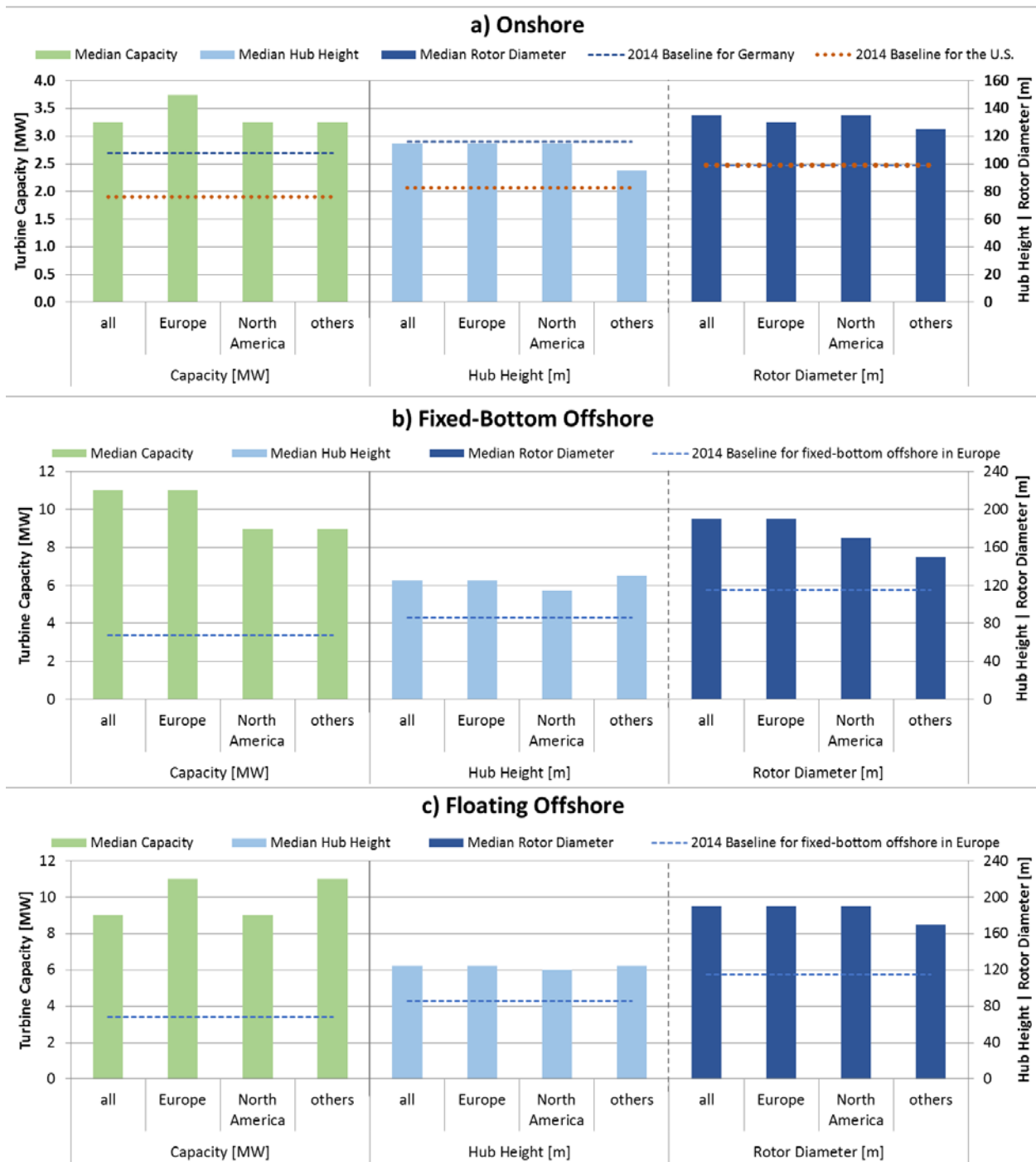
Figure 10. Wind Turbine Characteristics in 2030 for (a) Onshore, (b) Fixed-Bottom Offshore, and (c) Floating Offshore Wind Projects
