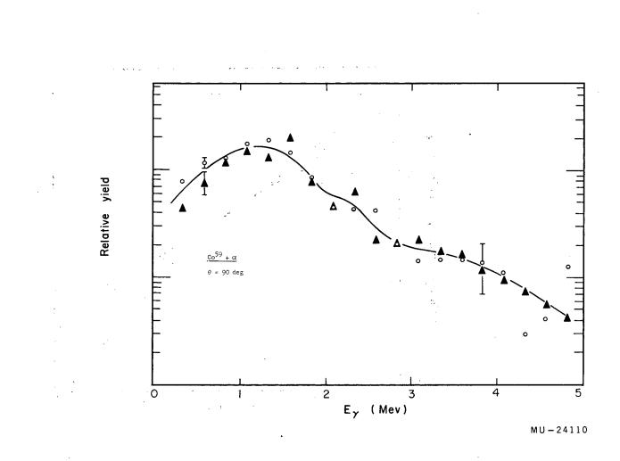
Fig. 8. Comparison of gamma spectra from alpha bombardments of cobalt at the two accelerators. Correction for detector response has been made. For  $\operatorname{Co}^{59} + \alpha$ ,  $\theta = 90$  deg, open circles show cyclotron points at  $\overline{E}^* = 46$  Mev; closed triangles show Hilac points at  $\overline{E}^* = 39$  Mev.
