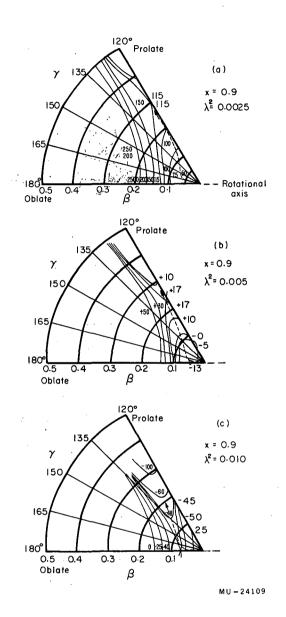
Fig. 1. Contour maps of the energy surface for a rotating nucleus. Energy contours are in units of  $10^{-5}E_s^{0}$ , where  $E_s^{0}$  is the surface energy for the spherical shape, and x = 0.9. Values of  $\lambda^2 \propto I^2$  are given on each map.
