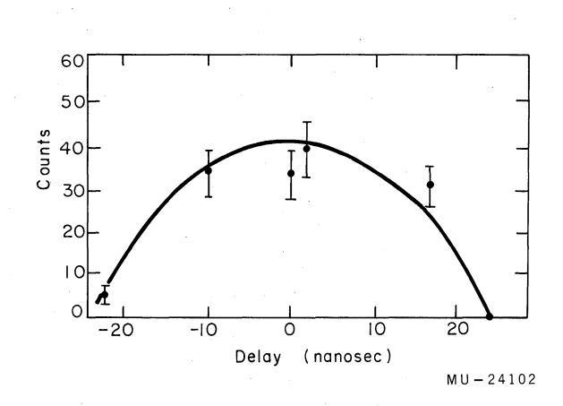
Fig. 5. Typical delay curve. The number of gamma ray counts is plotted as a function of the delay in Channel 3, with the other delays optimized with respect to that channel.
