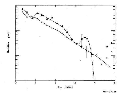
Fig. 19A. Spectra for alpha particles on Ba with  $\overline{E}^* = 42$  Mev. On curve with open circles,  $\Theta = 90$  deg; with closed triangles,  $\Theta = 45$  deg.
