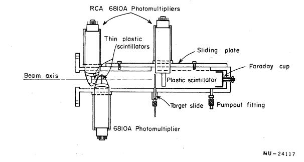
Fig. 2. Target and scintillator assembly. The stopping plastic scintillator may be moved relative to the target by means of the sliding plate.
