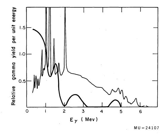
Fig. 22B. Comparison of gamma spectra for this experiment with spectra from thermal-neutron capture. As spherical nuclei,  $\text{Te} + C^{12}$  at  $\overline{E}^* = 99$  Mev (heavy line) is compared with thermal neutrons on tin (light line), since thermal neutron data for cerium are not available. Neutron capture data are from Groshev et al. (Ref. 84).
