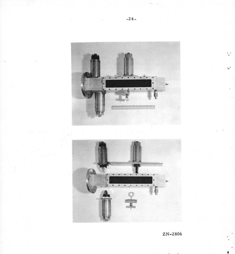
Fig. 3. Target and scintillator assembly: assembled (top) and disassembled (bottom) views, showing attachment of reflector frames to the photomultipliers. at the face of the crystal to  $1 \frac{1}{4}$ -in. at the side near the target minimized scattering by the collimator. This collimator was necessary to reduce the large peak caused by photons scattered in the shield.
