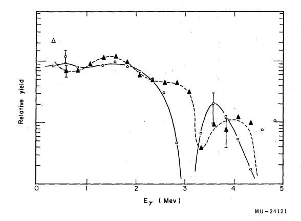
Fig. 16B. Comparison of gamma spectra for  $C^{12}$  on  $V^{51}$ , with  $\overline{E}^* = 49$  Mev. On curve with open circles,  $\theta = 90$  deg; with closed triangles,  $\theta = 45$  deg.
