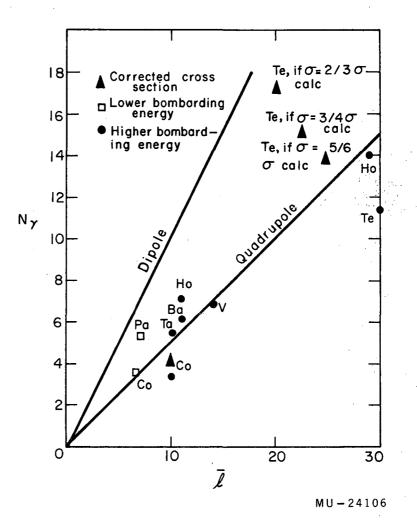
Fig. 21. Gamma ray yields  $n_{\gamma}$  as a function of the estimated average angular momentum  $\overline{\ell}$  at the start of the cascade. The dipole and quadrupole lines represent  $n_{\gamma} = \overline{\ell}$  and  $n_{\gamma} = 1/2 \overline{\ell}$ , respectively.
