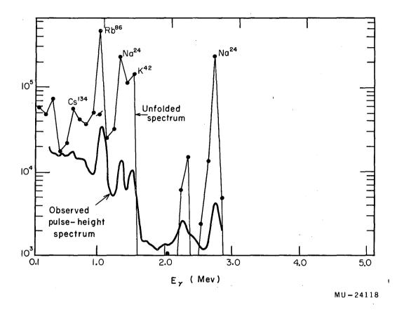
Fig. 12. Comparison of observed and unfolded spectra for a mixture of several sources:  $Rb^{86}$  at 1.06 Mev;  $Na^{24}$  at 1.38 and 2.75 Mev;  $K^{42}$  at 1.55 Mev; and  $Cs^{134}$  at 0.60 Mev.
