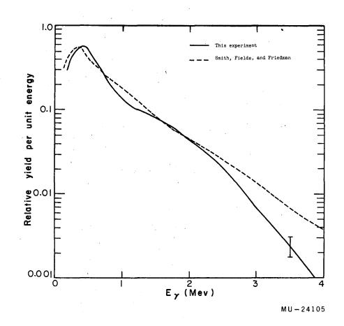
Fig. 7. Comparison of unfolded fission gamma-ray spectrum of Cf<sup>252</sup> with that obtained by Smith, Fields, and Friedman(Ref. 58).
