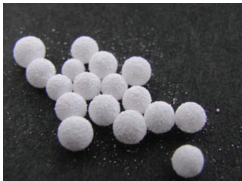
Figure 1.2: Photograph of liquid marbles about 1 mm in diameter (courtesy of S. Fujii, Osaka Institute of Technology, Japan).
