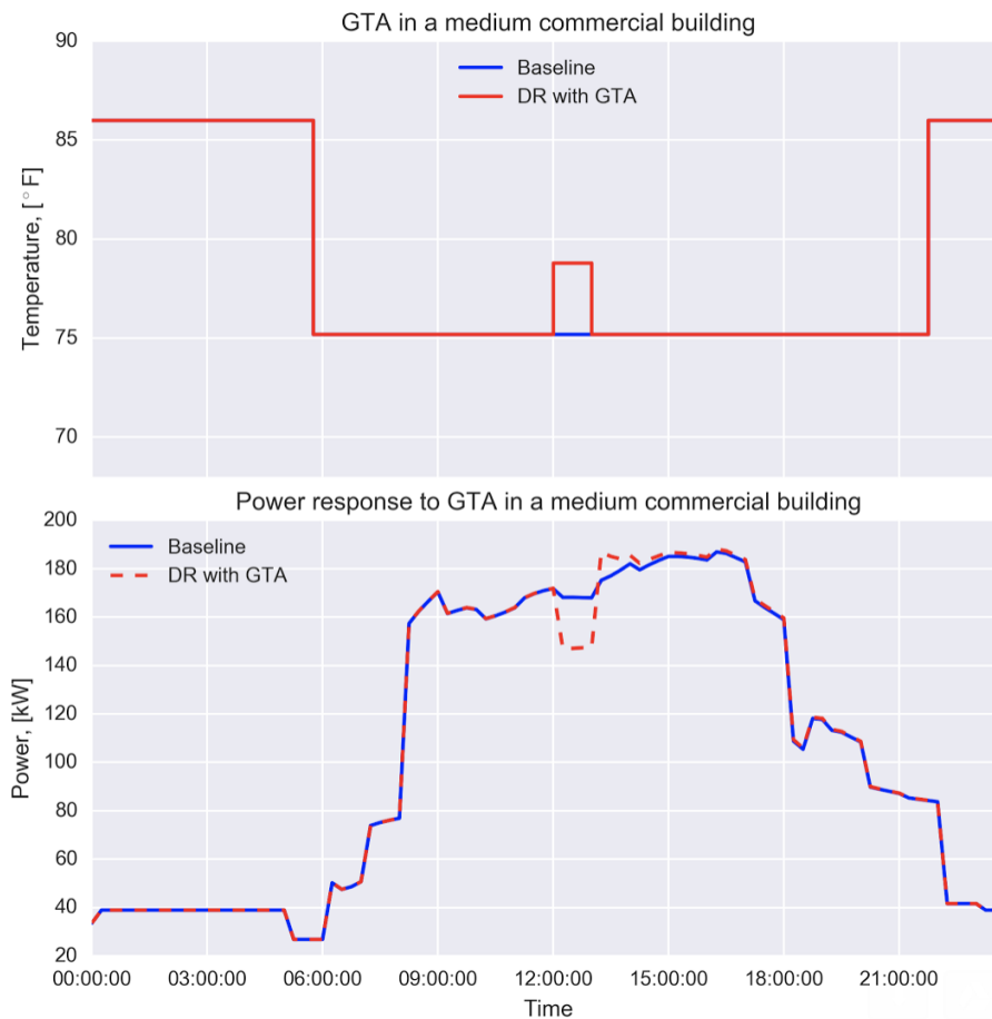
FIGURE C- 1. TEMPERATURE AND POWER IMPLICATIONS OF GTA IN MEDIUM COMMERCIAL BUILDING AS MODELED BY ENERGYPLUS
