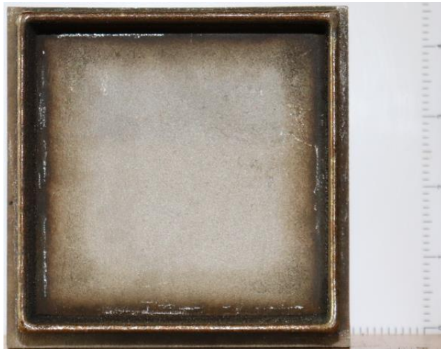
c) 100 mm square block with maximum cladding parameters
