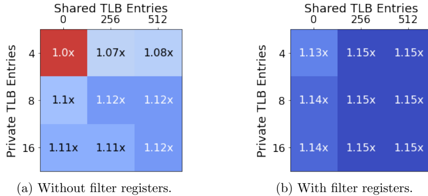
Figure 3.17: Normalized performance of ResNet50 inference on Gemmini-generated accelerator with different private and shared TLB sizes.
