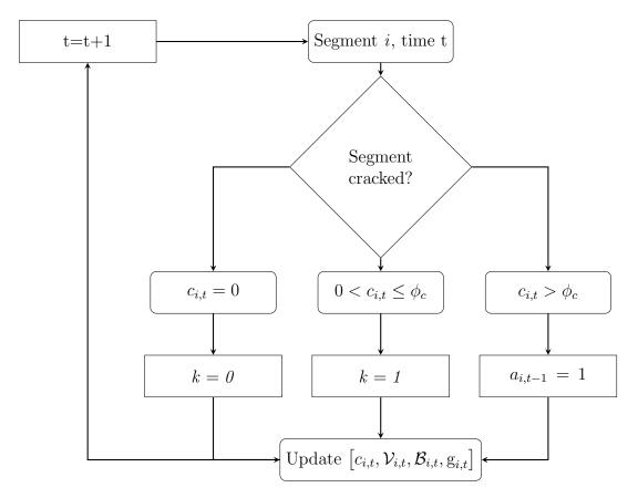
Figure 3.1: Illustration of the simulation process for a given pavement segment through one time period. The crack-initiation model is applied on a crack-free pavement segment. However, if cracking has initiated but has not reached the cracking threshold,  $\phi_c$ , the crack progression model is applied. On reaching the cracking threshold, an overlay action will be triggered which will simultaneously compute the resulting emissions and costs.
