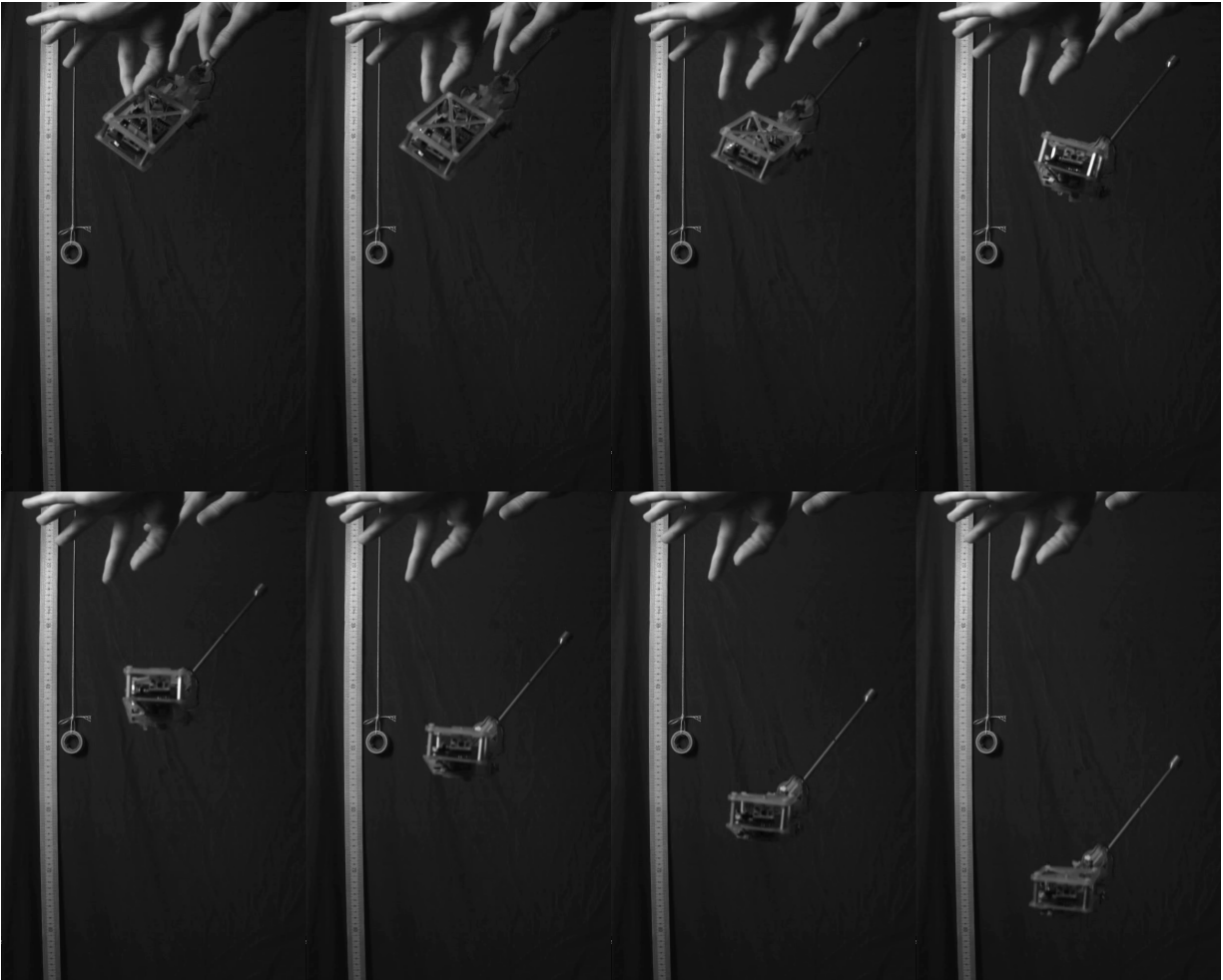
Figure 4.13: Sequence of frames during a correction in pitch, yaw, and roll. The desired orientation is pointing towards the reader.
