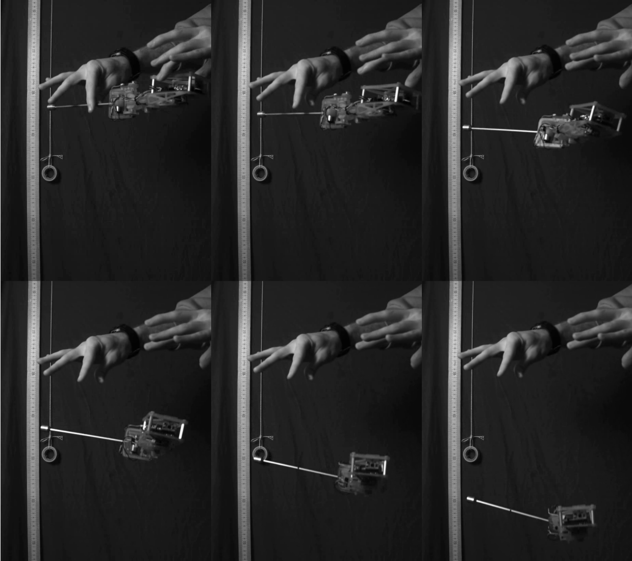
Figure 4.11: Sequence of frames during a pure yaw correction. The desired orientation is pointing towards the reader.
