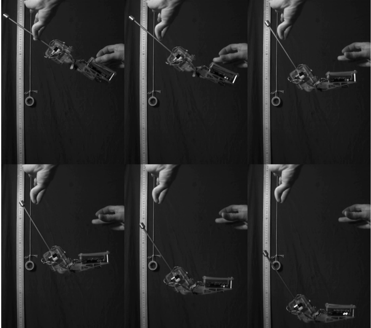
Figure 4.10: Sequence of frames during a pure pitch correction. The desired orientation is horizontal and pointing towards the right.
