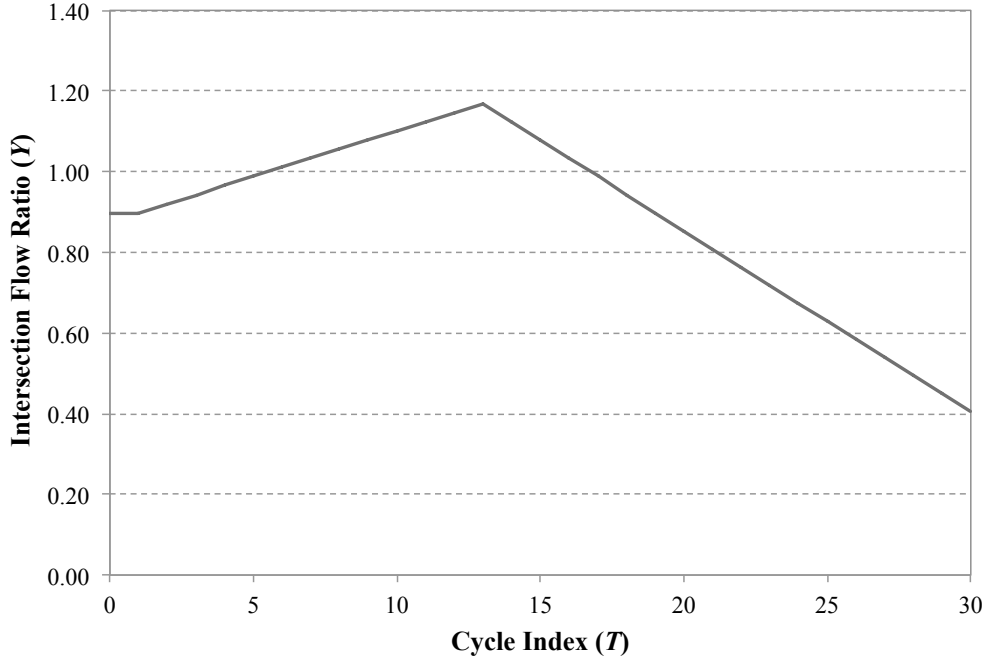
Figure 4.14. Intersection Flow Ratios for the 1 Hour Time-Dependent Demand Profile (Test Type II: Intersection of University and San Pablo)
