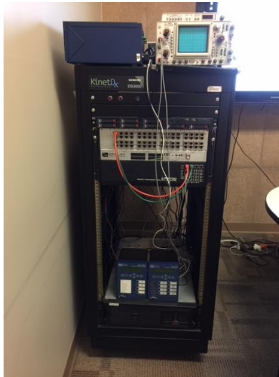
Figure 58. Controller RT-HIL testing setup.
