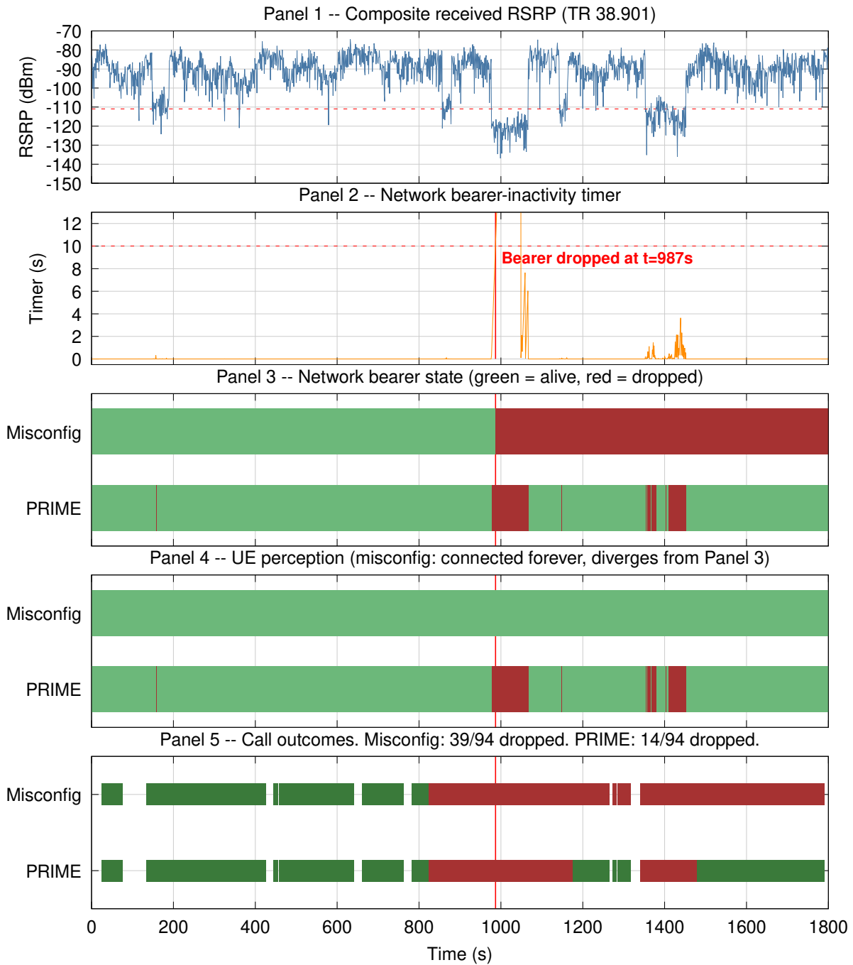
Figure 6.7. C5 (RLF detection). Without RadioLinkMonitoringConfig the UE never detects out-of-sync and its view of the connection diverges from the network's; enforcing RLM co-presence with the RLF timers restores out-of-sync detection and call recovery.
