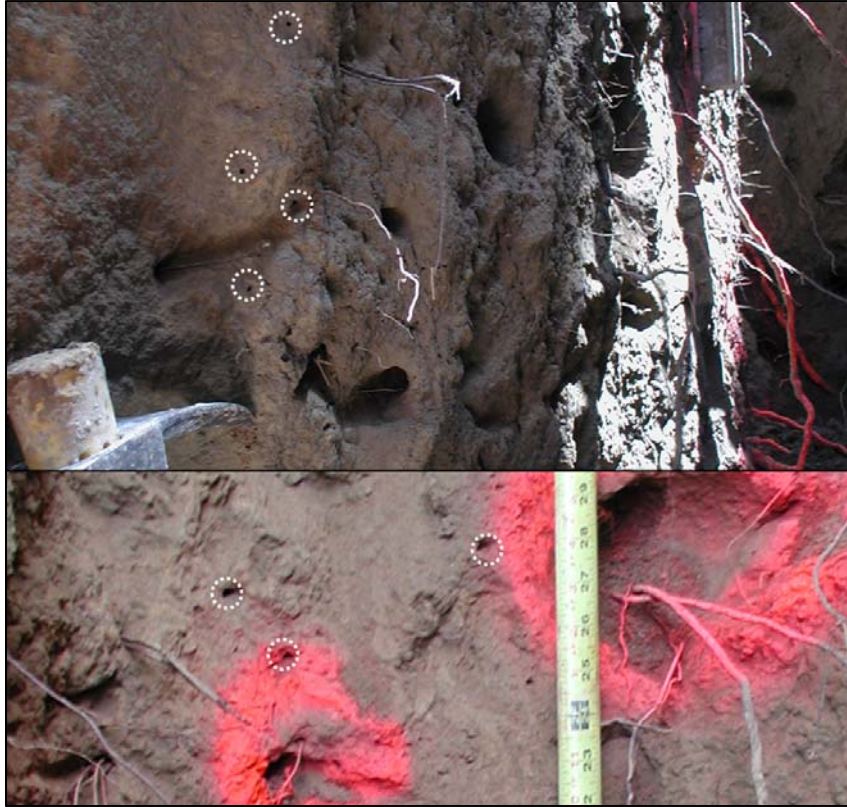
Figure 3-78. Small holes, less than 1/2 inch in diameter observed near mammal burrows.
