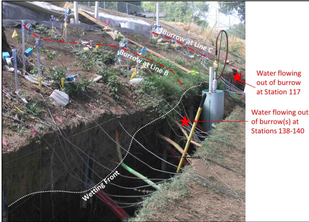
Figure 2-56. View looking west at the uphill wall of the lower stump trench 50 hours into the flow test. Gopher burrow outlet locations at Stations 138.25 and 117 are identified on the diagram as well as approximate alignments of burrows.
