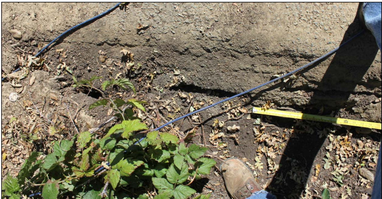
Figure 3-137. A blackberry bush is the transition point between the fresh crack (left) and an older crack (right).
