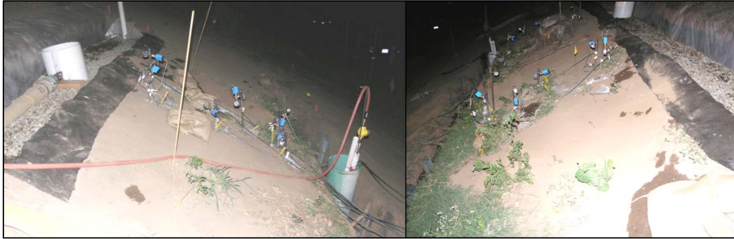
Figure 2-43. View of instrument line C (left) looking west and instrument Lines A and B looking east (right) 9.25 hours into the flow test. Note isolated seeps (darker spots) and gravel bags (covering seeps) at the top of Line C and extending down Line B.
