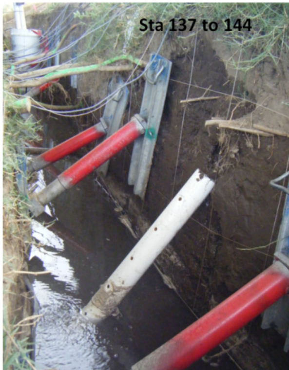
Figure 2-48. Saturation patterns in lower wall face at 29.1 hours after inundation of the upper trench with water. The lower stump (top left) and control (top right) trench wall seepage patterns are documented by station with corresponding photos below.
