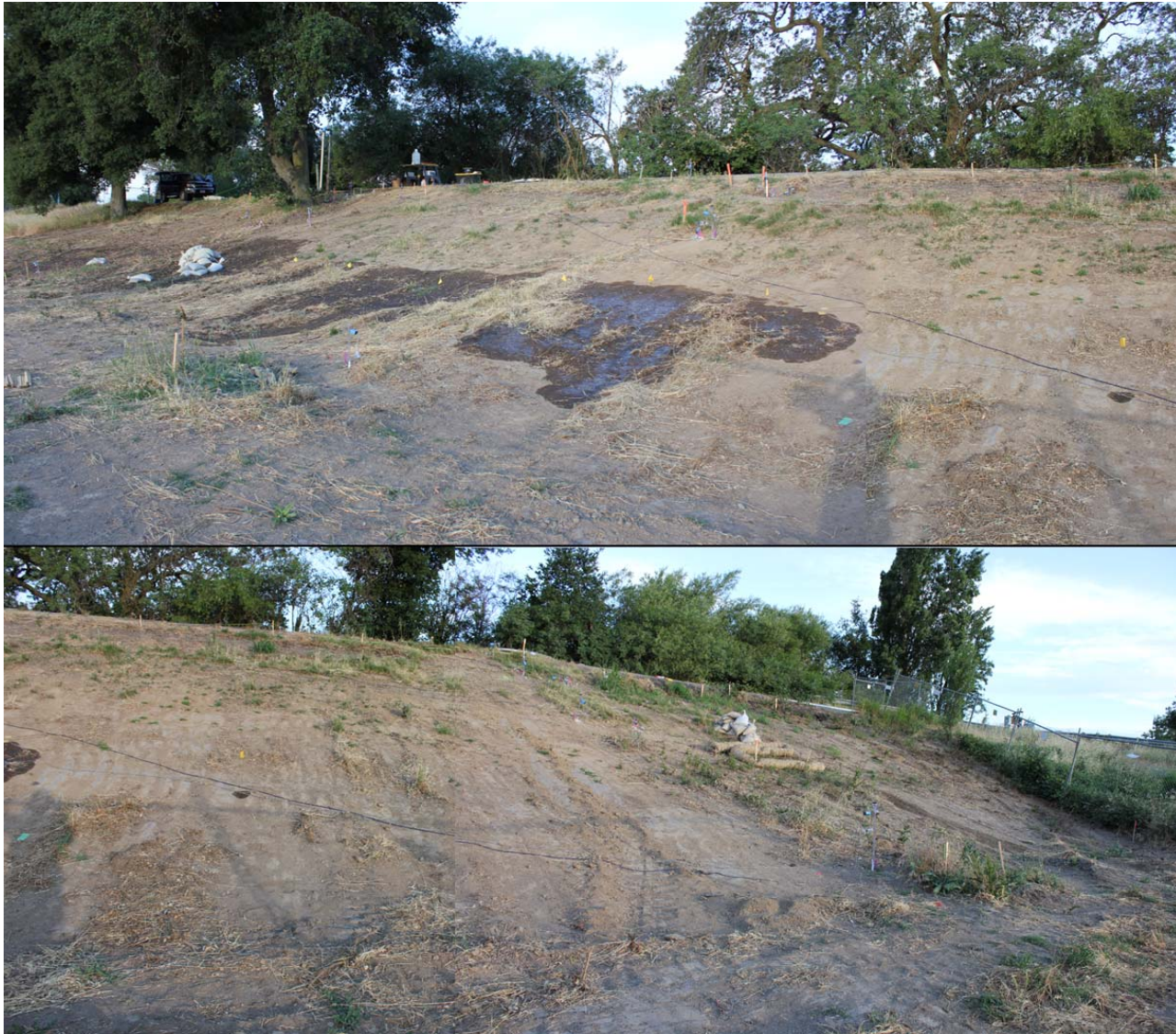
Figure 3-107. Time = 93 hours (6:45 am on 5/25/12); Small new seep near Station TT 3 while seeps to the south expand.
