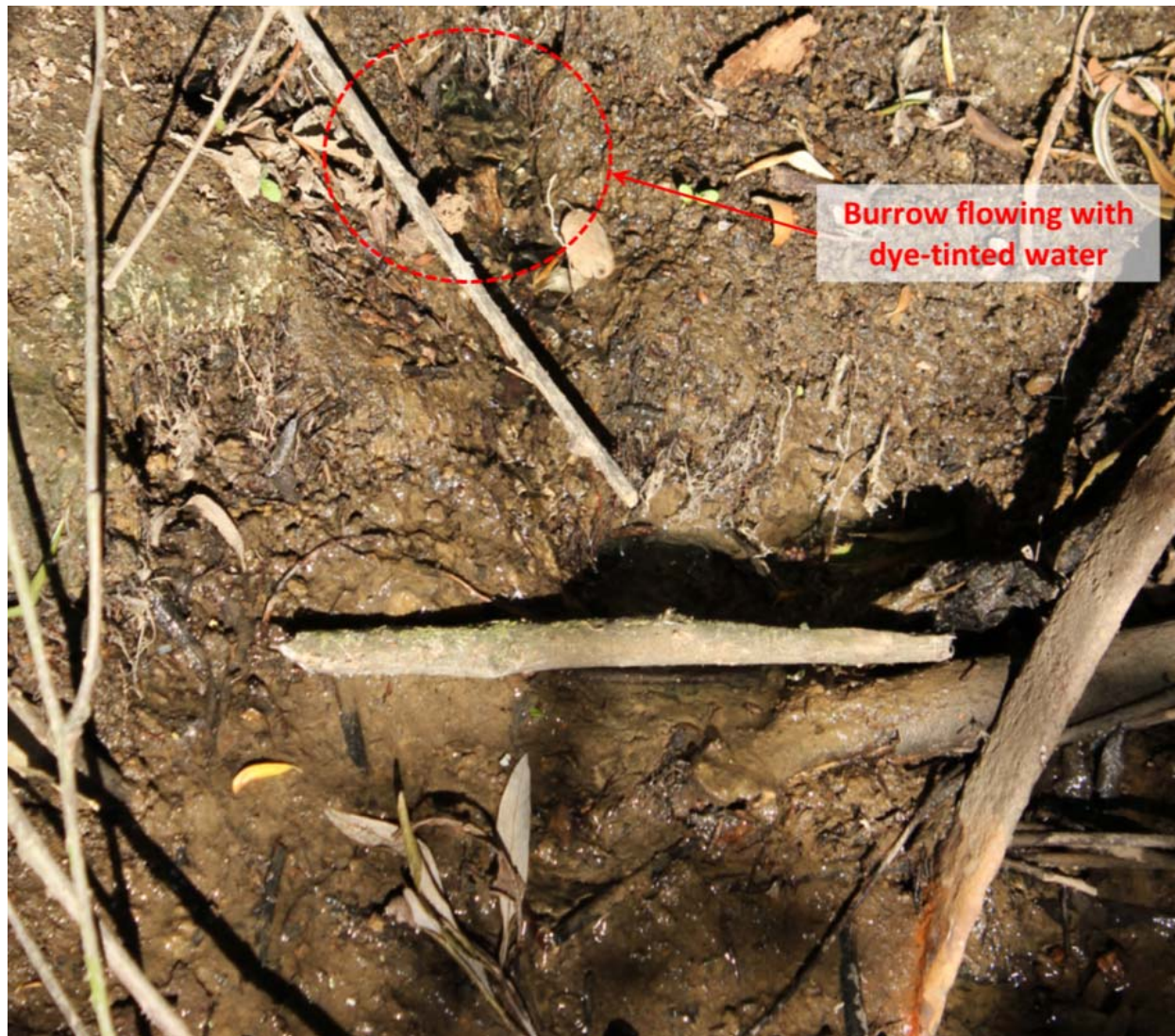
Figure 3-149. Burrow at Station TT 70 flows blue-tinted water at a measured rate of about ½ gallon per minute from a 2 ½ inch diameter burrow, likely muskrat.
