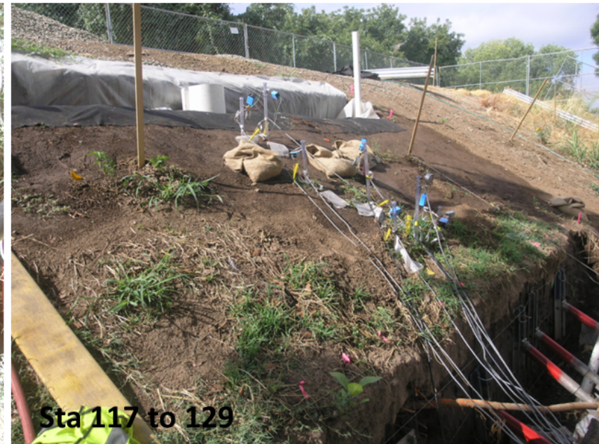
Figure 2-51. Saturation patterns in lower wall face at 46.6 hours after inundation. Note the depression in the saturation pattern in the area of the decomposed root at Station 147. The lower stump (top left) and control (top right) trench wall seepage patterns are documented by station with corresponding photos below.
