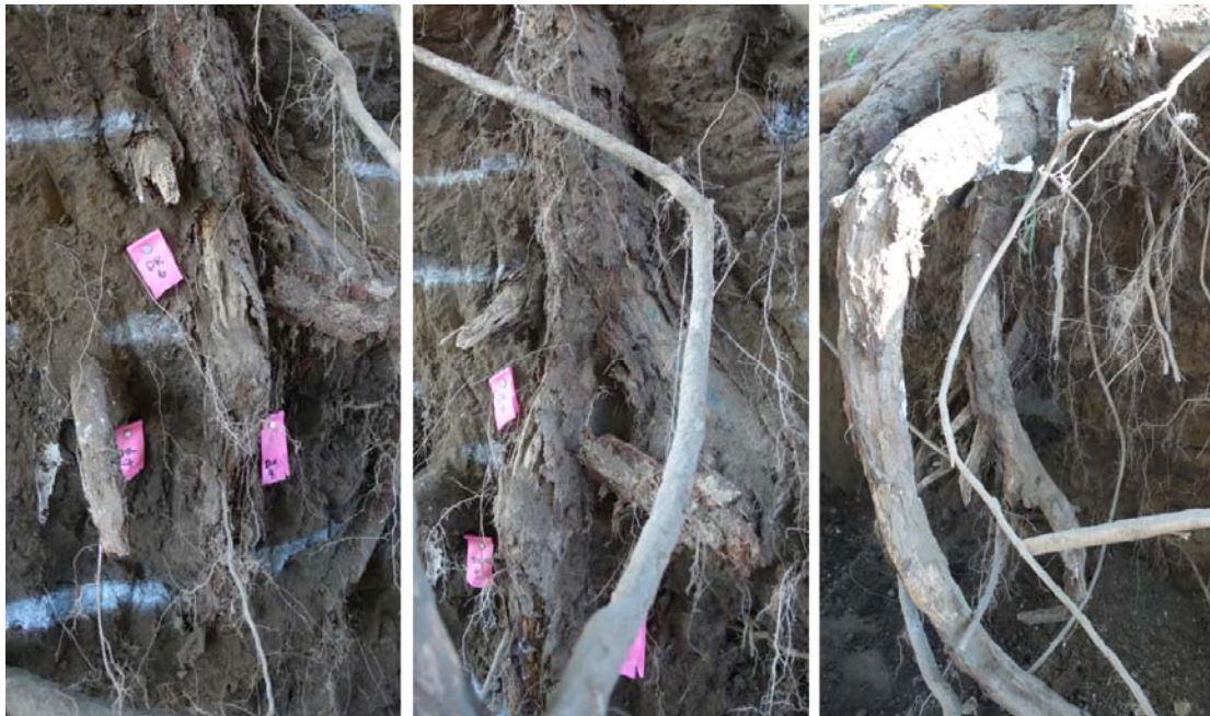
Figure 2-83. Typical appearance of decomposing roots encountered. Bark was fragile and discontinuous in many places. Annular spaces are seen on larger roots. Photos by Richard Evans.
