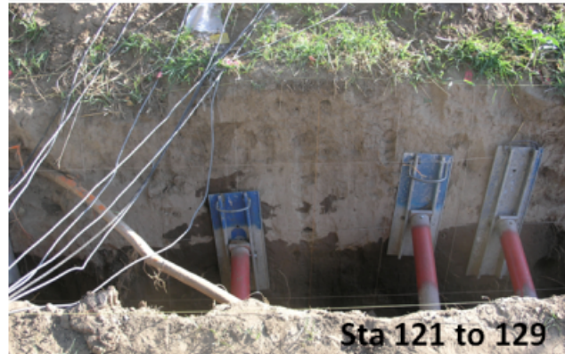
Figure 2-48. Saturation patterns in lower wall face at 29.1 hours after inundation of the upper trench with water. The lower stump (top left) and control (top right) trench wall seepage patterns are documented by station with corresponding photos below.
