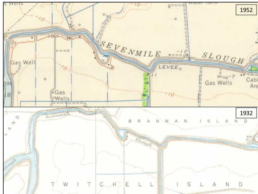
Figure 3-9. Historic topographic maps: USGS (1932) and USGS (1952). Note the position of structures have changed along the Sevenmile Slough between 1932 and 1952. A flow control gate has been installed by 1952 and the oxbow section appears to be wetland.
