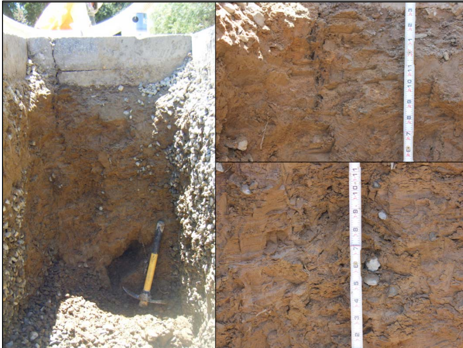
Figure 3-175. View looking south at the upper 4 feet of control trench end wall at Station CT 31.5 (left) with close-in views of cracking near the top of the trench (upper right) and just above and to the left of the burrow.
