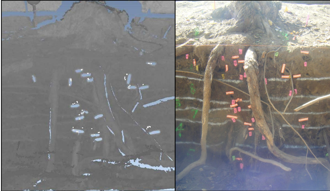
Figure 2-98. Slice 1 comparison between T-LiDAR image (left) and photograph (right). Note reflectors in T-LiDAR image indicating burrows (vertically oriented) and decomposing roots (horizontally oriented). Source: Cobos-Roa et al. 2012.
