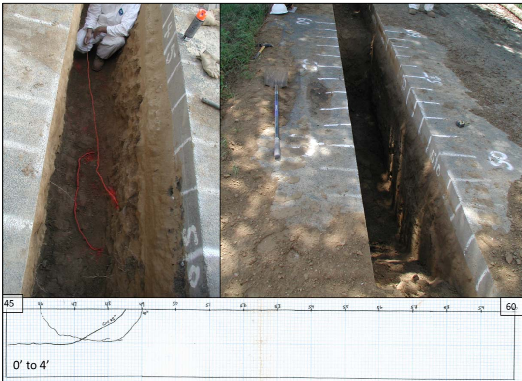
Figure 3-58. Root log at 0 to 4 foot depth Station TT 45 to 60.
