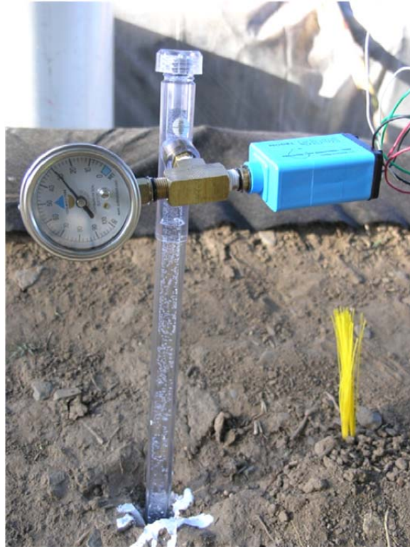
Figure 2-40. A typical tensiometer is shown including a mechanical gauge and pressure transducer. White silica sealing material is seen at the hole entrance.
