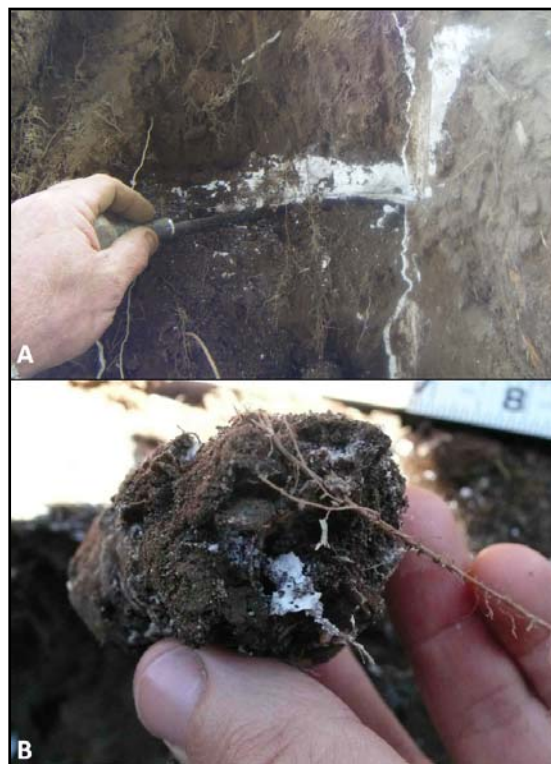
Figure 2-87. Silica slurry freely flowed in burrows (as shown in A) and void spaces within roots (as shown in B) when a direct hydraulic connection was available (or present).
