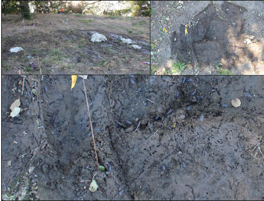
Figure 3-174. Gravel bag Station 73 below landside oak tree. Pill bugs seemed to disappear into a cavity that, upon excavation, did not seem to extend anywhere or resemble a burrow. Worm traces were found to be abundant as in other locations.
