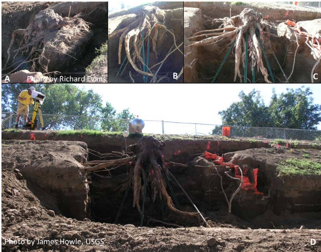
Figure 2-93. View of stump excavation following removal of ‘Slice 3’ soils. Photo A is a view of the stump from the crest of the levee looking down into the upper trench. Photos B through D show the stump from varying angles. Photo D also shows T-LiDAR scanning in progress.
