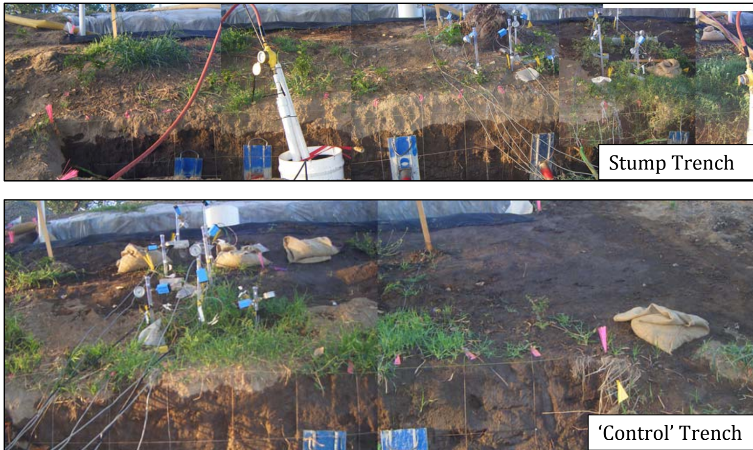
Figure 2-54. Saturation patterns in the stump and control trenches at 140 hours into the flow test, just before the end of the test. Only small changes were observed in saturation patterns between 67.9 hours and 140 hours.
