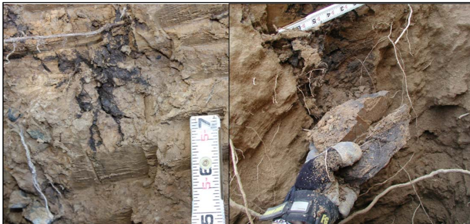
Figure 3-49. Materials 1 and 3 (left) and Material 2 (right) exhibit manganese oxide staining on what appear to be fractures within the levee soils.
