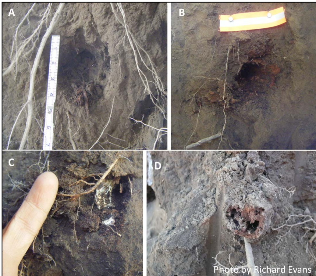
Figure 2-89. Roots can leave a void where they become completely decomposed and surrounding soils and live roots have not yet in filled the void. The root in Photo D has likely been subjected to decomposition from biological activity.
