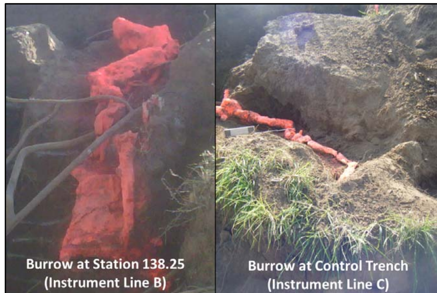
Figure 2-75. Mammal burrows at instrument Lines B and C following post-flow grouting and characterization efforts.
