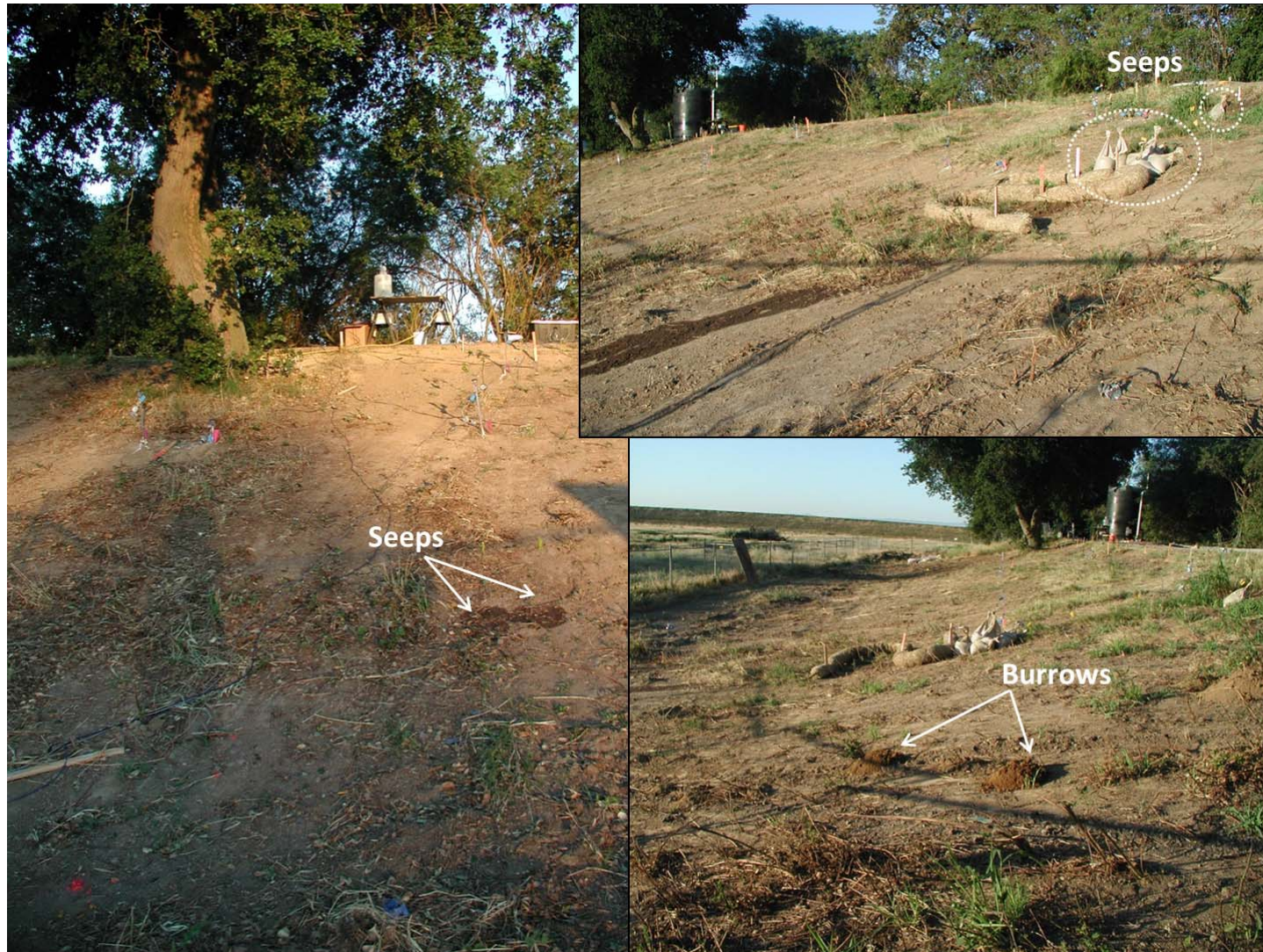
Figure 3-98. Time = 15.8 hours (5:30 am 5/22/13): Seeps at Line D (left), macropore flow near Line C (top right), and active gopher activity to north of control line (lower right).
