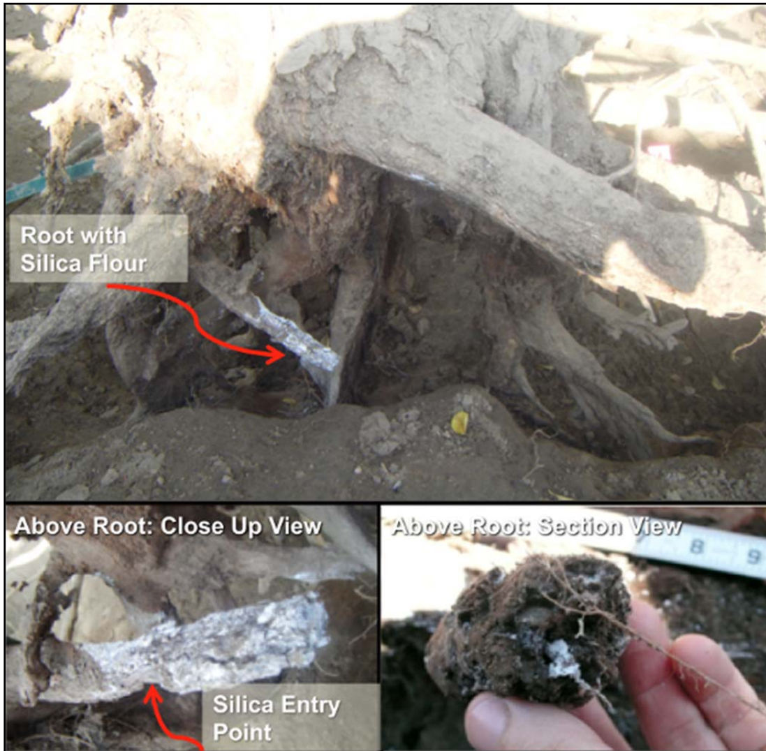
Figure 2-94. View root system of the decomposing stump looking north from the upper trench (top). Note migration of silica flour through a path directly traceable to a location where the installation of a tensiometer penetrated the root.
