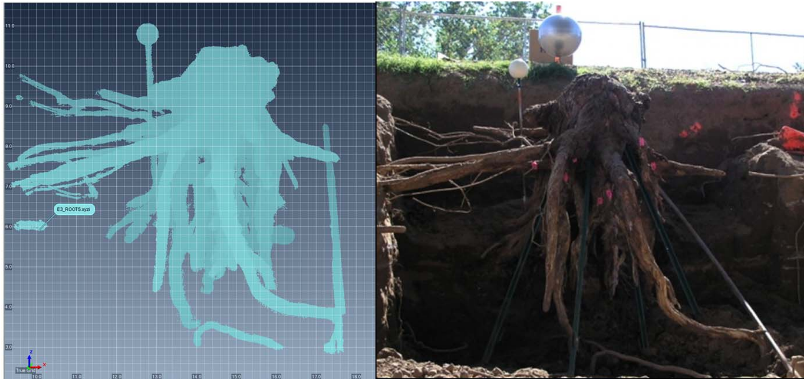
Figure 2-103. A south-facing view of eucalyptus stump and root system (right) and the corresponding point cloud image (left) derived from combining data from a series of T-LiDAR scans. T-LiDAR image courtesy of Gerald Bawden of the USGS.
