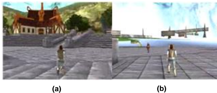
Figure 3.1. Comparison of video frame quality for different rendering setting with 300kbps bit rate: (a) view distance = 150m; (b) view distance = 70m.
