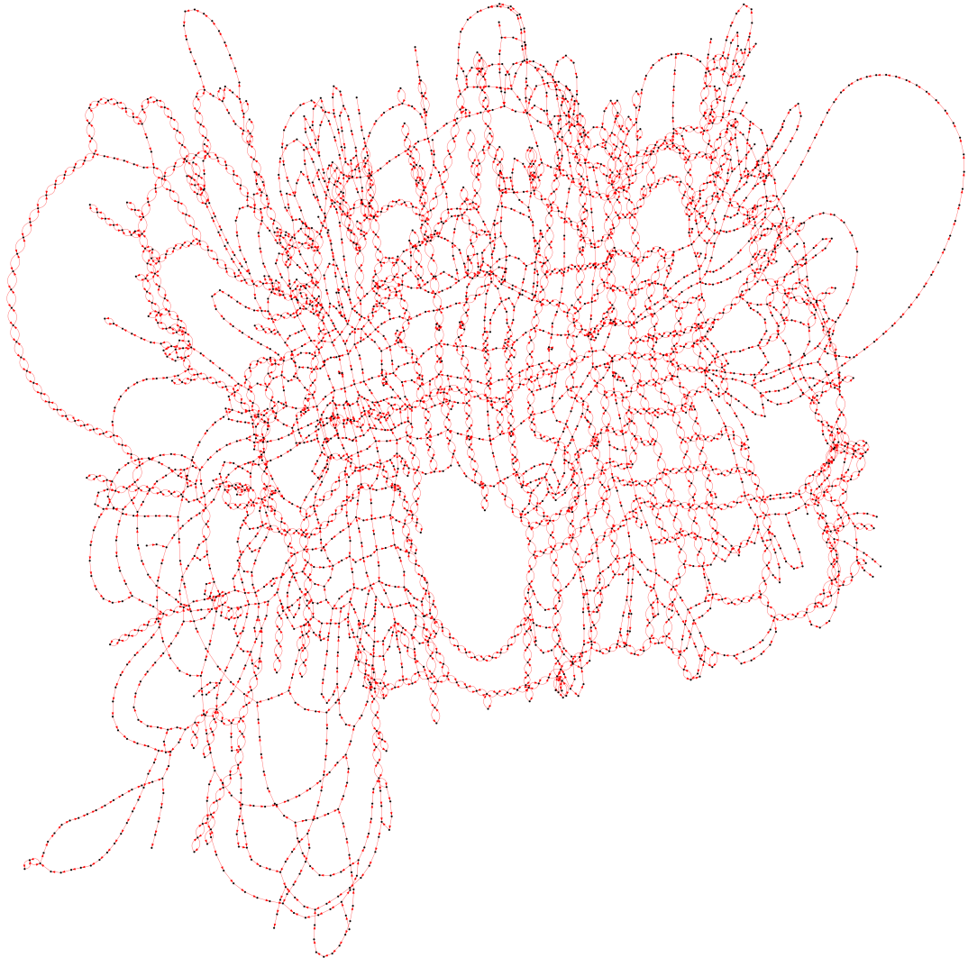
Figure 2.4: Graph of the region of Washington D.C. using Kamada Kawai layout [KK89]. Vertices are black and edges/arrows (indicating direction) are red. Representation mainly serves to depict connectivity; the locations of the vertices in this image are loosely based on their corresponding true relative locations, but the edge lengths are not to scale.
