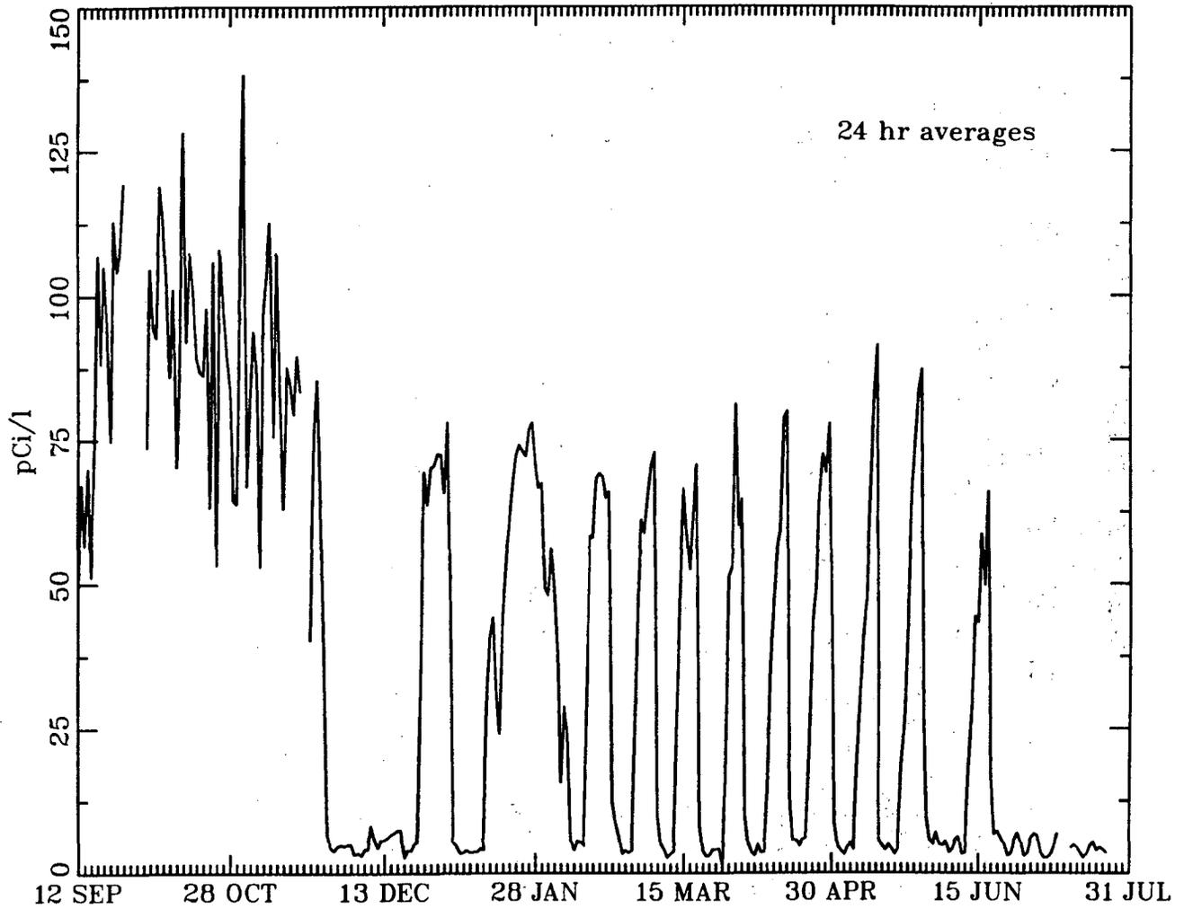
Figure 4. Basement radon levels from September 12, 1986 through July 1987 for house LBL12. The data have been averaged over 24 hours. The periodic spikes are due to the weekly cycling of the SSV mitigation system which began February 23 and continued through June 25, 1987.
