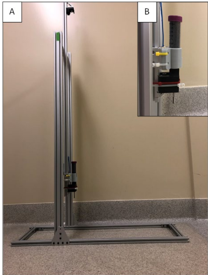
Figure 2 - Weight drop injury apparatus A. full side view of weight drop rail B. close view of weight sitting atop stopper with hex bolt pushed through
