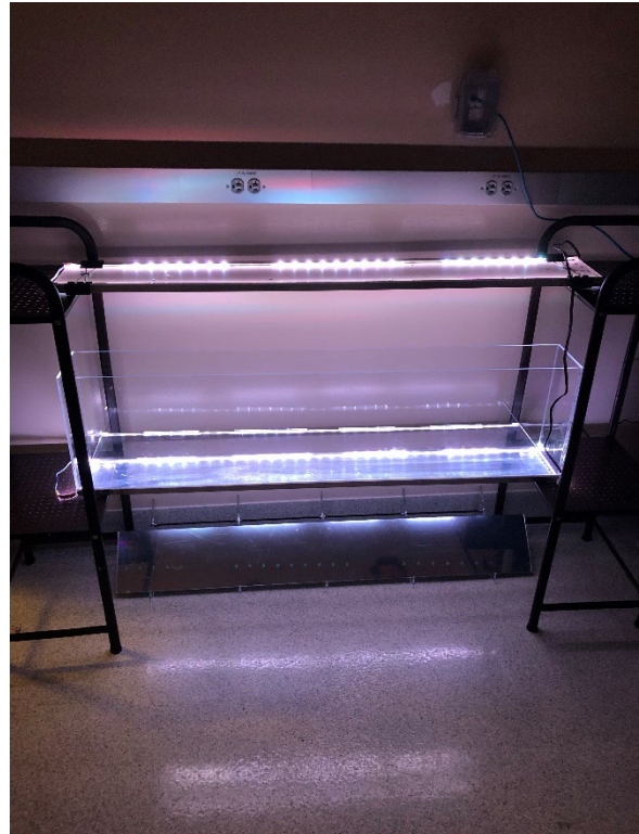
Figure 11 - Gait analysis walkway with acrylic arena installed and LED lights turned on. The mirror sitting underneath the walkway is elevated to just under the walkway during testing but is positioned on the floor here for ease of view.
