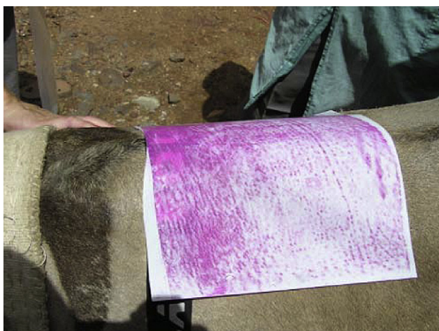
Figure 5 Extreme low pressure 4 LW Fujifilm showing higher-intensity results. This film was used with a cart with 400 kg of maize (corn) loaded on it. The film shows pink concentrated in the front, near the withers.
