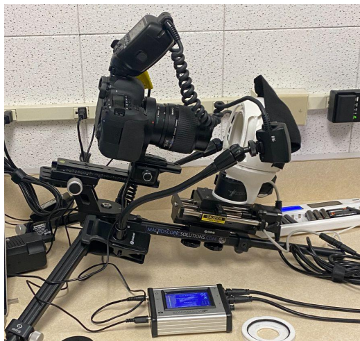
Fig. 3: Camera and stage setup for focus-stacking
