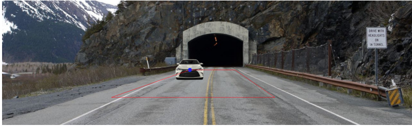
Figure 5.6. Annotation trapezoid. User adjusts the four corners that represent the valid sampling subspace of x and z . The size of the car scales according to how close it is to the vanishing point.
