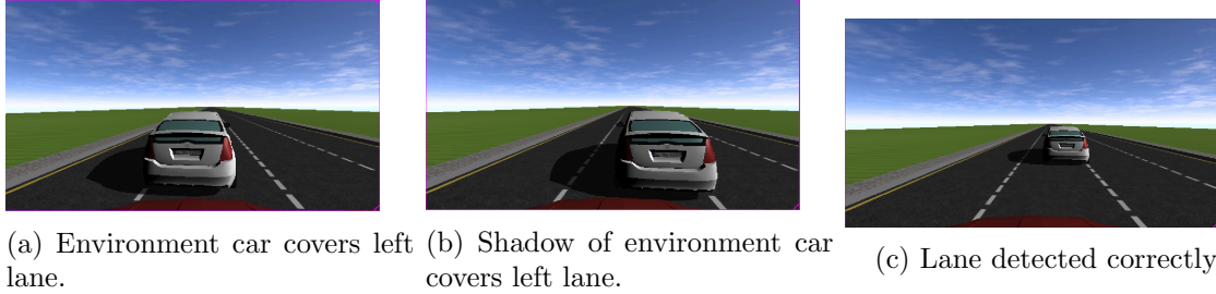
Figure 7.7. The lane detection fails for (a) and (b) and \mathcal{S} car tries to slow down. When lane is correctly detected (c), the LQR controller tries to follow the lane
