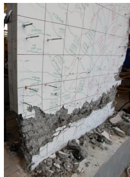
Fig. 8-4—Out-of-plane instability and concrete crushing of a wall test reported by Dashti et. (2018).
