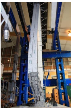
Fig. 8-4—Out-of-plane instability and concrete crushing of a wall test reported by Dashti et. (2018).
