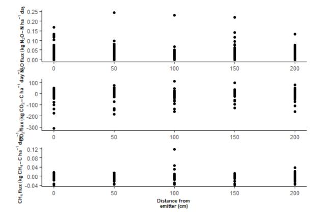
**Figure 2.14:** Gas fluxes (top: N<sub>2</sub>O, middle: CO<sub>2</sub>, bottom: CH<sub>4</sub>) from all sampling collars relative to the distance (cm) the collar was placed from the fan jet micro-sprinkler emitter.
