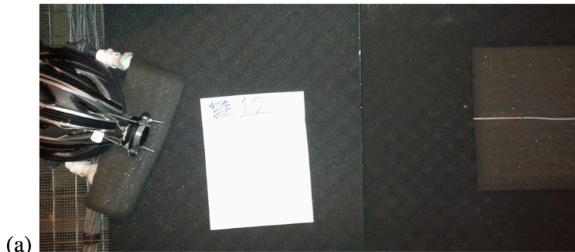
Fig. 6.3 Measurement of transfer functions for ultrasonic microphones and ultrasonic speaker as a function of angle. (a) Angular transfer function measurement setup. (b) Angular transfer function data. For the microphone, the sensitivity relative to the sensitivity at zero degrees is plotted; for the speaker, the emission power relative to the emission power at zero degrees is plotted.
