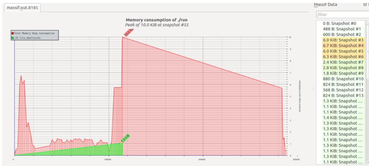
Figure 5.3: First Layer memory profiling
