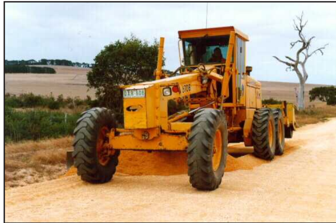
Figure 1. A Caterpillar grader, which is commonly used for roadworks in southern NSW.
