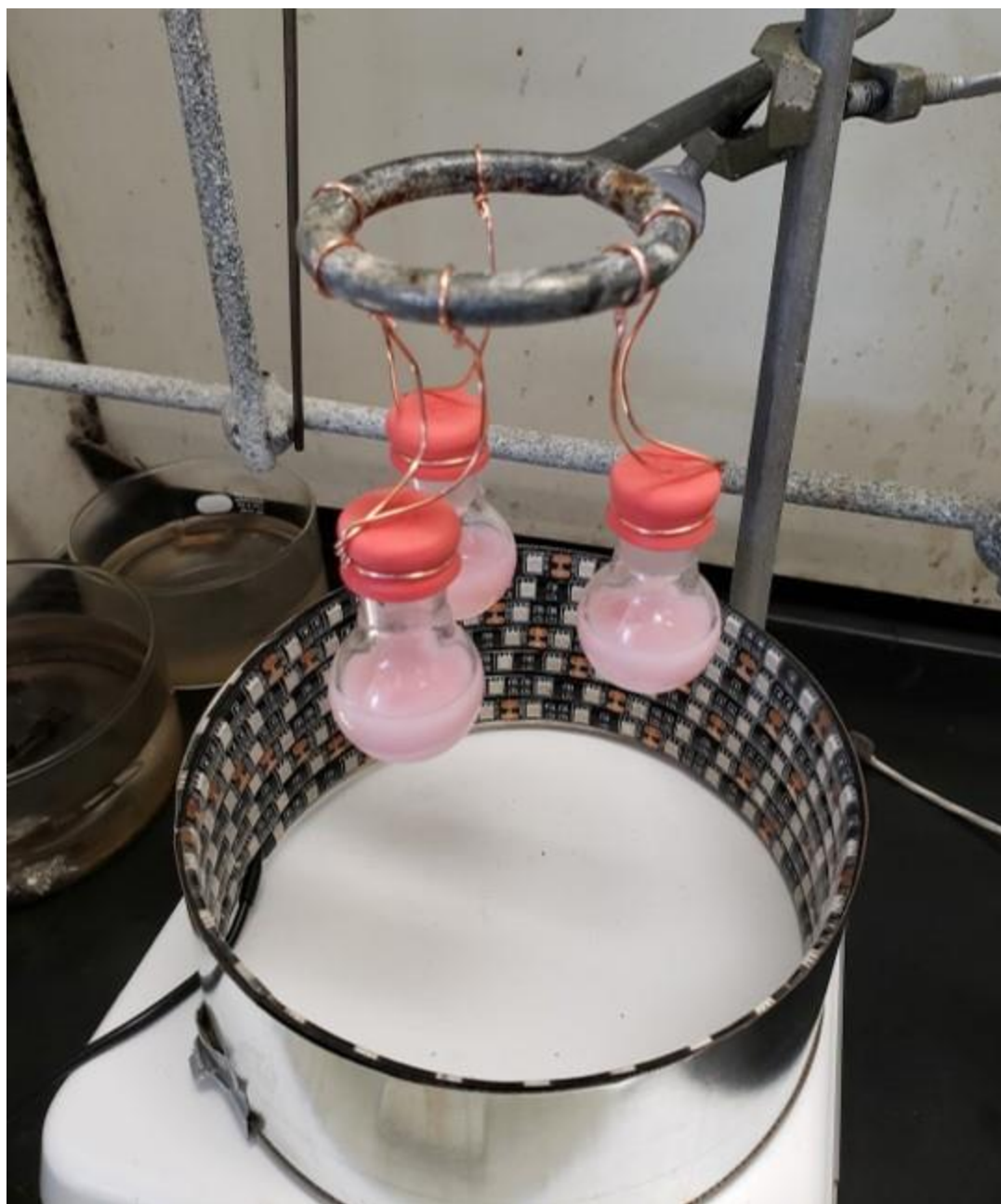
Figure 3S.4. Home built LED reaction vessel lined with blue led strips.
