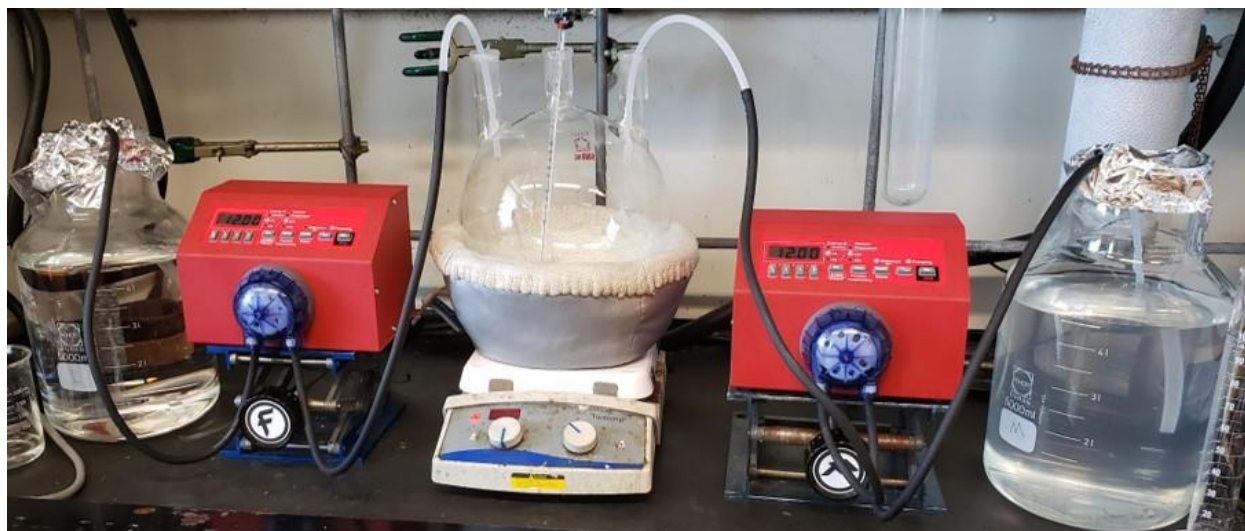
Figure 3S.1. Experimental setup for the large- scale synthesis of UiO-66 x . 4L Flasks (left and right sides) contain separate stock solutions of H 2 bdc and ZrOCl 2 ·8H 2 O in DMF (30 mM). Peristaltic pumps deliver both solutions at prescribed feed rates to the 4L 3-neck round bottom flask set in a heating mantel. The mantel was used to hold the temperature of the reaction solution at 120 °C.
