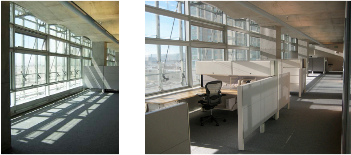
Figure 4.6 Examples of depth of direct sun penetration on the SE facade during Phase 2 (left: September 2, 11:15 AM PST) and Phase 5 (right: November 9, 8:30 AM PST). Images are taken from areas of the SFFB that were unoccupied during the study.
