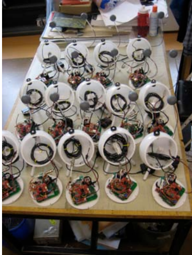
Figure 4.32 Final assembly and inspection of polling stations (left) and operational reliability testing (right).
