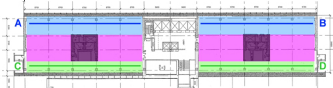
Figure 10.1 Typical tower floor plan showing location of 4 perimeter photo-controlled lighting zones (NW = blue, SE = green). Interior zones (purple) varied by floor. Blue and green horizontal lines indicate location of overhead luminaires.
