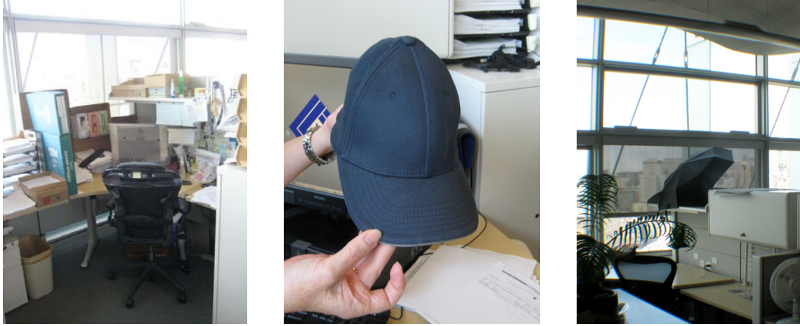
Figure 11.6 Examples of interior workspace modifications to control direct sun and reduce window luminance observed in the NW perimeter zones.
