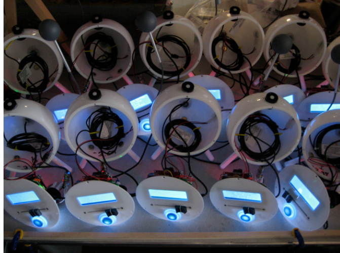
Figure 4.32 Final assembly and inspection of polling stations (left) and operational reliability testing (right).
