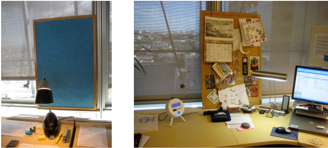
Figure 10.11 Examples of supplemental task lighting added to SE workspaces where the facade was shaded by ad-hoc opaque devices (e.g. bulletin boards).
