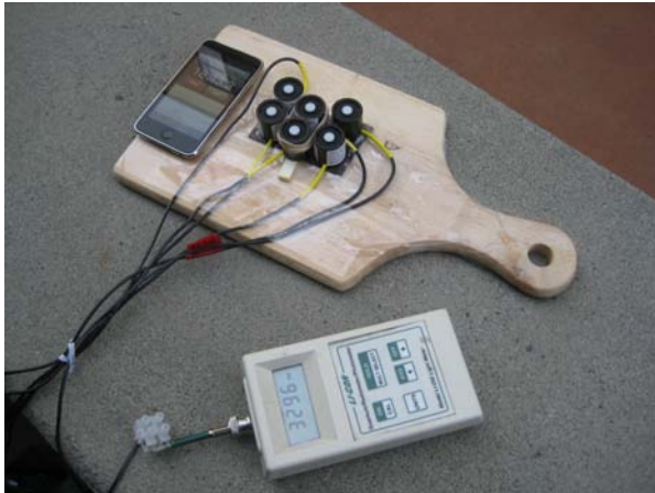
Figure A.5 Five LI-COR illuminance sensors calibrated using a reference LI-COR illuminance sensor connected to a LI-COR LI-250 light meter.
