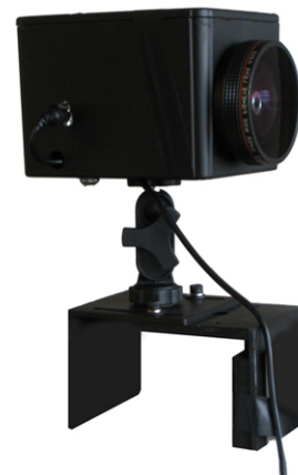
Figure 4.12 Typical placement of digital camera on SE facade perimeter zone workstation partition (left) and isolated view of device showing method of attachment (right). The camera's center of view was aligned perpendicular to the facade.
