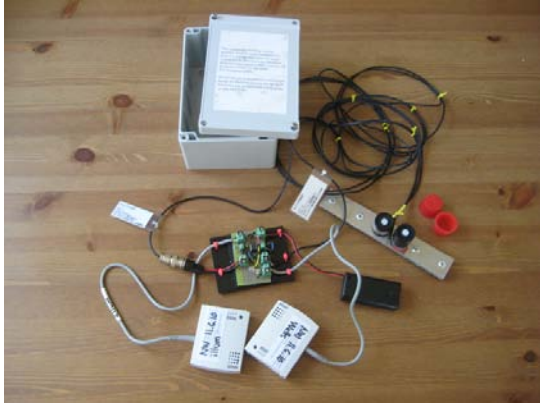
Figure A.3 Exterior illuminance and irradiance measurement and data logging device (left) and dual op-amp circuit (right).
