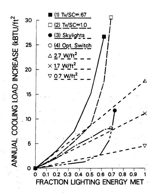
Figure 1: Annual cooling load increases as a function of the fractional lighting energy met from four fenestration systems and three electric lighting power densities in a prototypical office module in Lake Charles, LA. The required illuminance is 50 fc; vertical glazing is west facing.
