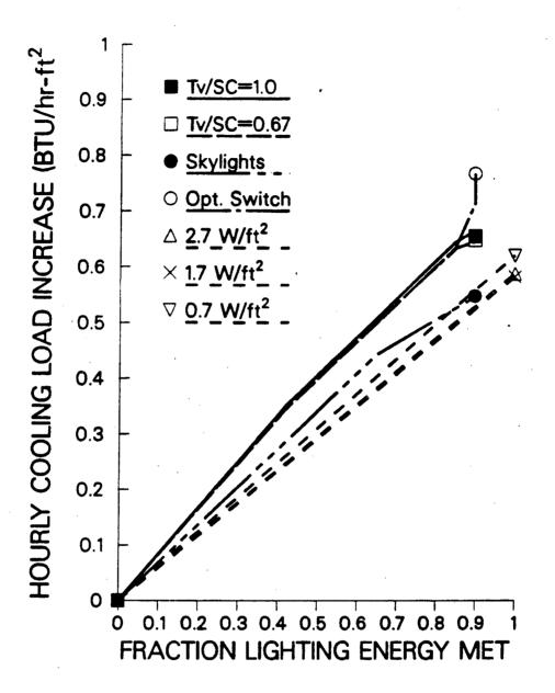
Figure 4: Peak hour cooling load increases normalized by the daylight coolness index as a function of the fractional lighting energy met from four fenestration systems and three electric lighting power densities in a prototypical office module in Lake Charles, LA. The required illuminance is 50 fc; vertical glazing is west facing.
