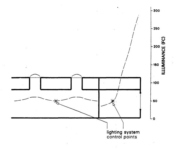
Figure 2: Daylighting illuminance distribution within both sidelighted and toplighted spaces for the peak hour in Lake Charles, LA. Apertures were sized to provide 50 fc at the lighting system control points. Vertical glazing is west facing. No shading devices are considered.
