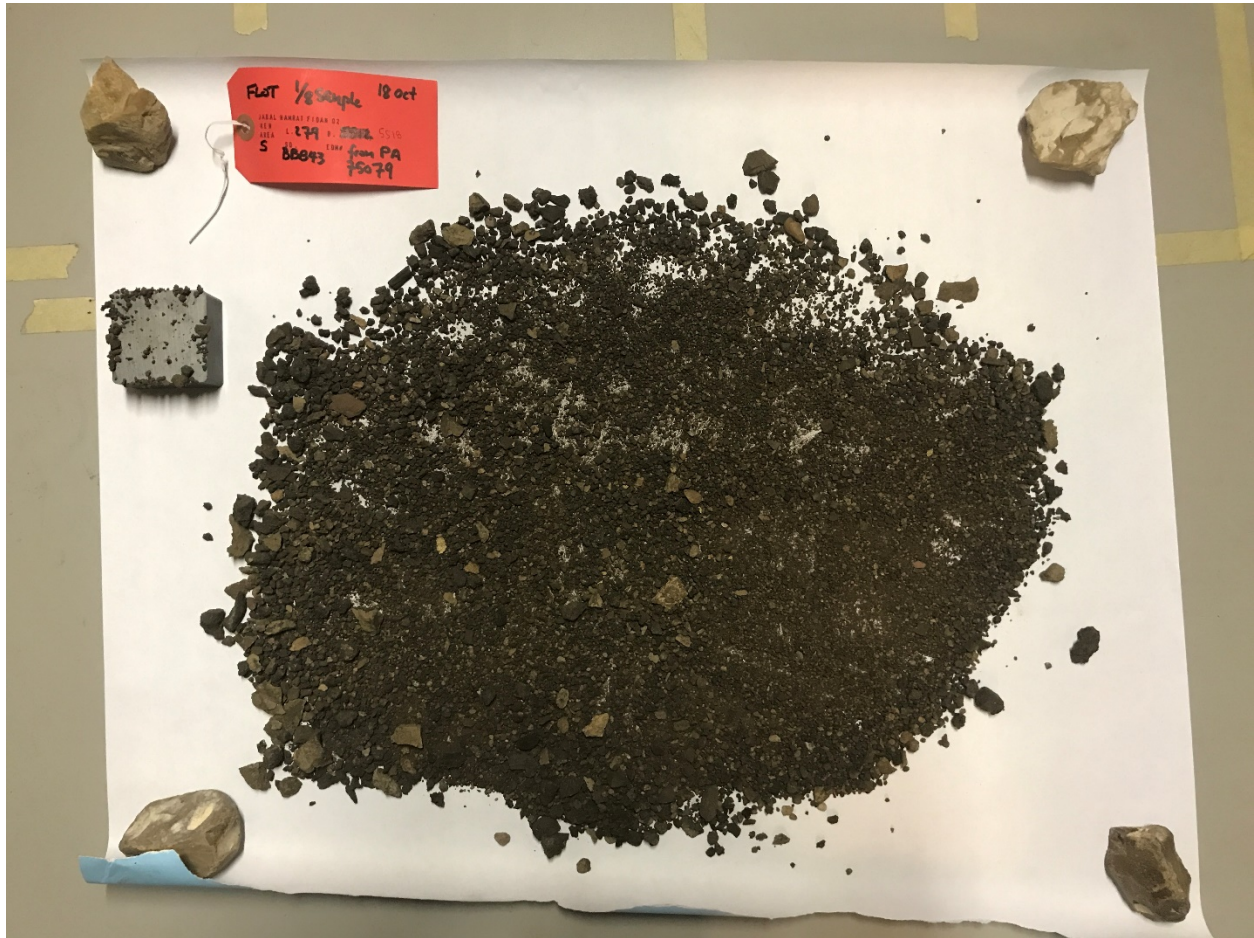
Figure 5.12: Methodology for collecting magnetic material from a sediment sample. The sample is spread into a thin layer and the magnet is dragged through the sediment to collect any magnetic material (some collected material is visible on the magnet – black square in the top left corner). Photograph credit: Brady Liss, UCSD Levantine and Cyber Archaeology Lab.
