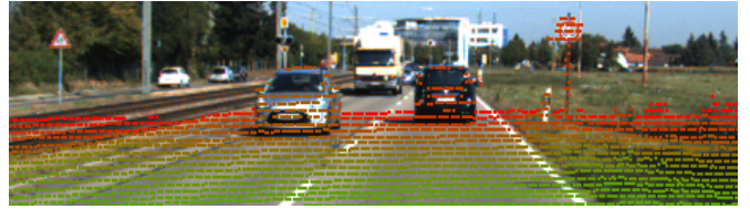
(a) Laser points projected on image. Color encodes distance.
