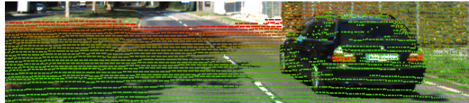
(a) 3D LiDAR point clouds projected on the image
