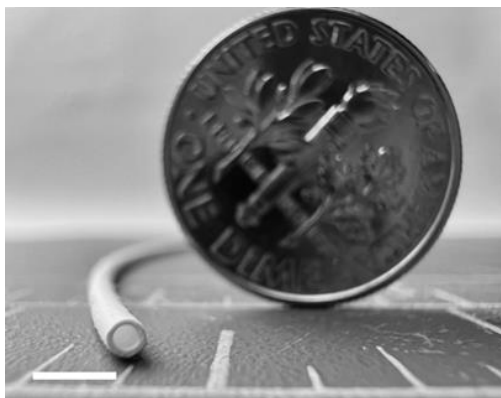
Figure 6. Electrospun DEVG is compared to a dime. The diameter of the DEVG can be tuned during electrospinning. The scale bar denotes a length scale of 5 mm.
