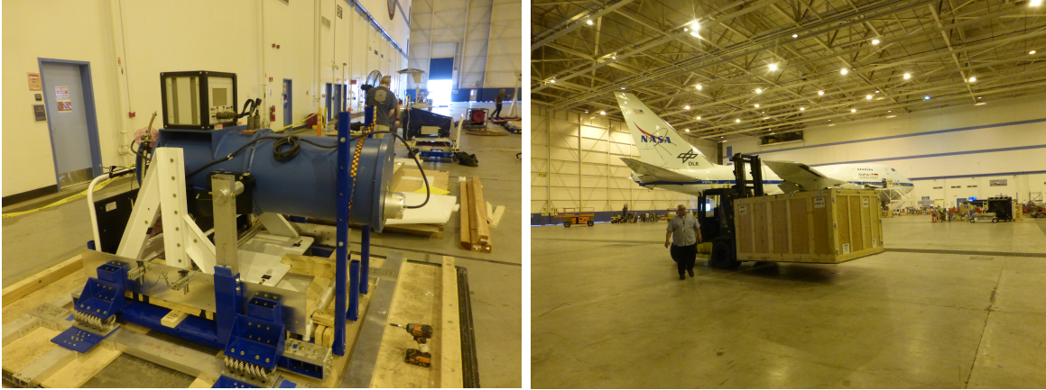
Figure 3.7 Left: The FLITECAM cryostat and handling cart mounted in their custom-built shipping fixture. Note the large isolator springs designed to protect against physical shock to the instrument. Right: The FLITECAM crate moving through the SOFIA hangar to be loaded onto the truck that will deliver it to LAX for shipment to New Zealand.
