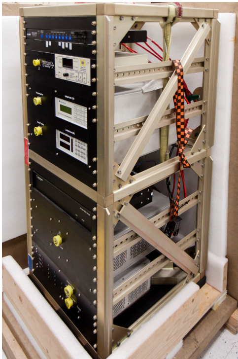
Figure 3.8 Left: The FLITECAM counterweight rack (CWR) undergoing a fit check in its foam-lined crate. Right: The FLITECAM CWR (left) and accessory pallet (right). Here I am investigating the CWR manifest attached to the side of the box.
