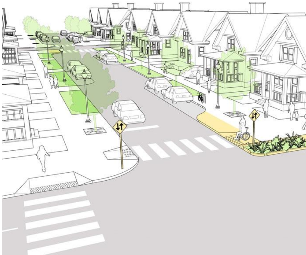
Figure 29. NACTO Recommendations for Yield Street (From Urban Street Design Guide , by NACTO, pp. 17).
