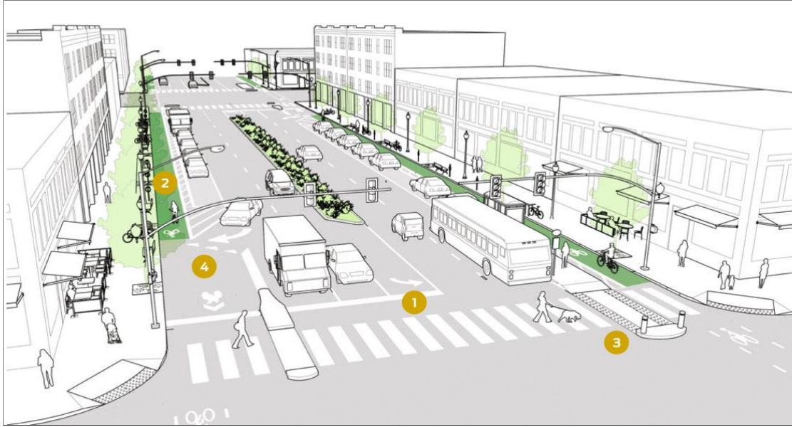
Figure 51. NACTO Recommendation for Major Arterial Street (From Urban Street Design Guide , by NACTO, pp. 13).
