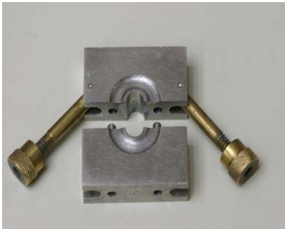
Figure 2. Disassembled mould apparatus displaying the two halves of the metallic mould used for confinement of cement samples during placement and setting
