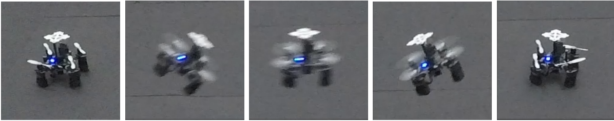
Figure 6.1: Video sequences of a quadcopter doing a short hop flight. The state estimation error of inertial navigation can be reduced significantly by breaking a long time flight into multiple short time hop flights.
