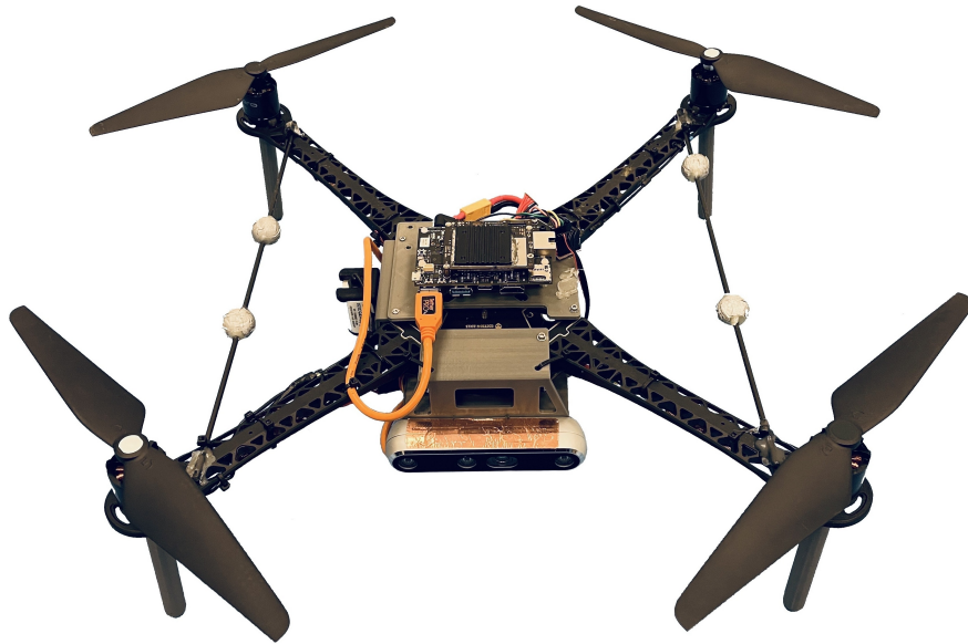
Figure 1.1: A custom-built quadcopter with motion capture marker balls and a stereo camera.
