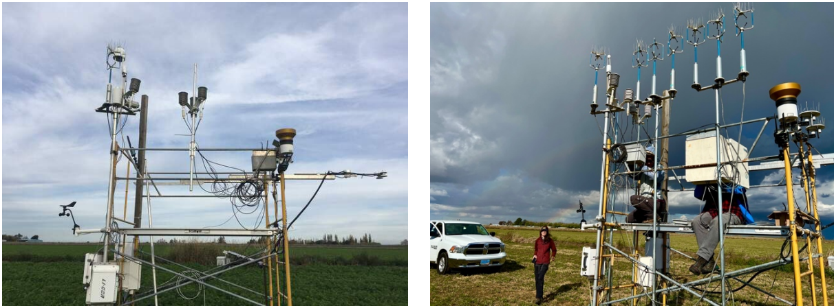
Figure H1. Examples of the side-by-side intercomparison for temperature and relative humidity sensors used in 2021 (left) and sonic anemometers used in 2022 (right).
