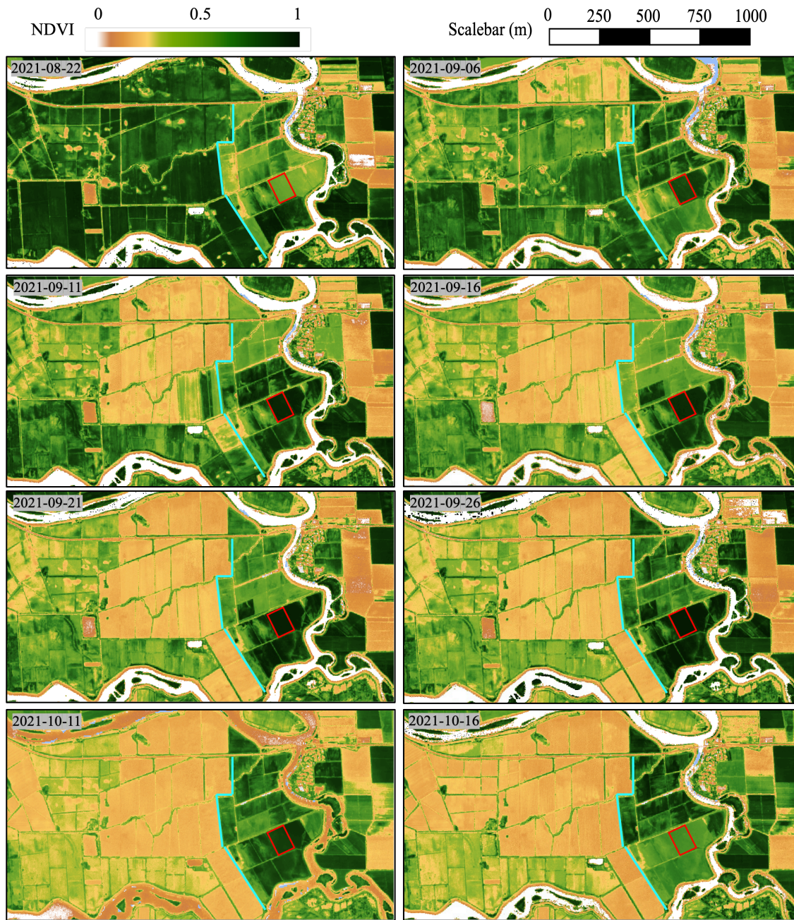
Figure 1. 2A. NDVI scenes (10 m) during the study period showing the dynamics of the vegetation status for by the alfalfa site (red) and its the upwind fields. The cyan colored line separates the upwind boundary with alfalfa fields on its right and corn fields on its left. All scenes were generated using Sentinel-2 (surface reflectance) on Google Earth Engine.
