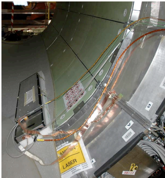
Figure C.2: Shown in this picture is the RIB in its position in the ECAL bore in the experimental cavern at P5.
