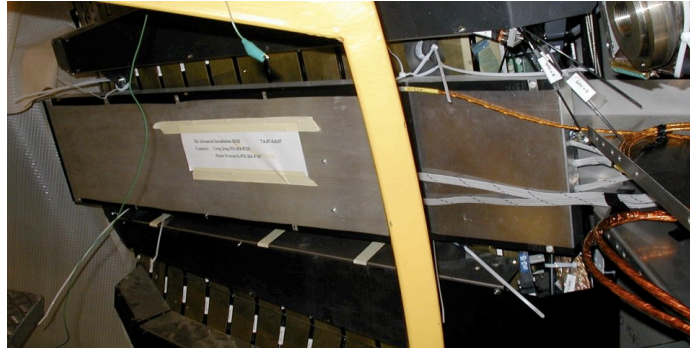
Figure C.1: Shown in this picture is the RIB in its position on top of a HCAL wedge in the experimental cavern at P5.
