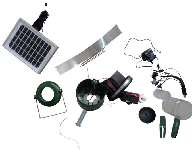
Disassembled powerpoint solar powered lantern.
