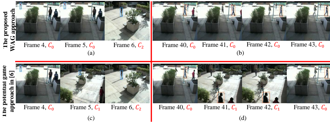
Figure 4.4: Experiment #1. Example frames for comparing smoothness during camera handoffs. The left column ((a) and (c)) corresponds to the left red ellipse in Figure 4.5 while the right column ((b) and (d)) corresponds to the right red ellipse in Figure 4.5. The first row is the result by using the proposed weakly acyclic game (WAG) approach while the second row is the result by using the potential game approach in Chapter 3. For easy observation, we only draw the bounding box for the person under discussion in the text. Person 4: the left column. Person 5: the right column. The red number at the left bottom is the ID of the camera that is assigned to track the person.
