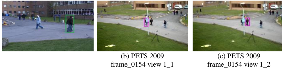
Figure 5.4: Necessity of tracker re-initialization with feet test. In (a) The system incorrectly decides that view 5 is the best camera view to track the occluded person based on the metrics. If there is no feet test, this error will propagate by using the front person’s position to re-initialize the tracker for the occluded person in view 1, as shown in (b). However, with a feet test, we know that there is a heavy occlusion and avoid the tracker re-initialization in view 1, as shown in (c). (Different colors are for different trackers.)
