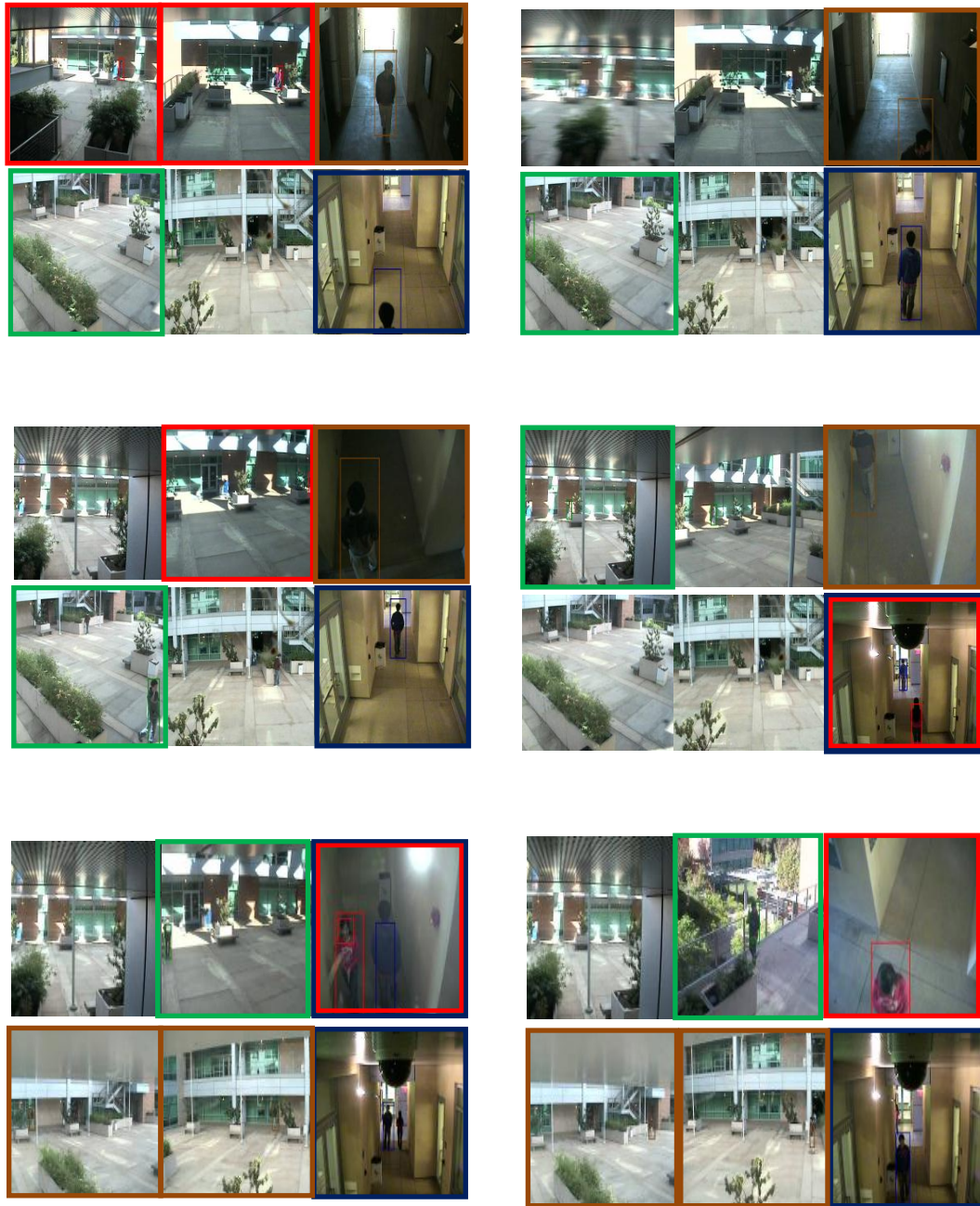
Figure 6.7: Experimental results in the 6 cameras 4 persons case. The camera images from the cameras in the same group for a person are boxed in the same color as the person they are assigned to follow.
