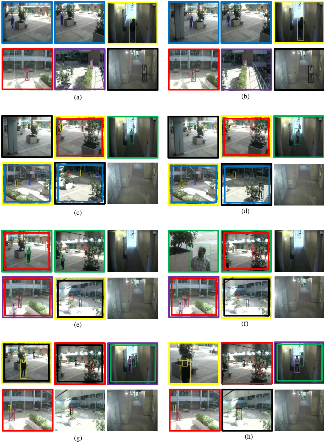
Figure 6.8: Experimental results in the 6 cameras 6 persons case. The camera images from the cameras in the same group for a person are boxed in the same color as the person they are assigned to follow.
