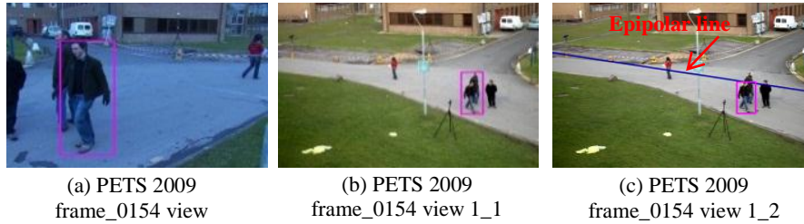
Figure 5.5: Necessity of tracker re-initialization with homography only and with epipolar geometry. (a) Selected view using online boosting. (b) Particle filter tracker re-initialization without providing the epipolar line. The re-initialized tracker in (b) still includes other person in it, which is a mistake. (c) The re-initialized tracker by using homography and epipolar geometry together avoids the problem in (b). Only a single person is in the bounding box.
