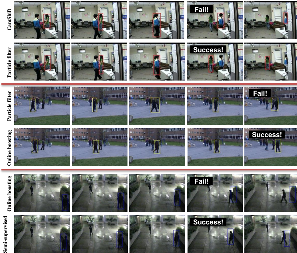
Figure 5.1: No single tracker is good enough for all scenarios. The first two rows show a scenario where the CamShift [18] tracker fails but the particle filter tracker [52] works well. The middle two rows show a scenario where the particle filter tracker [52] fails but the online boosting tracker [57] works well. The bottom two rows show a scenario where the online boosting tracker [57] fails but the semi-supervised online boosting tracker [58] works well. The failure and successful frames are marked as shown in the figure.
