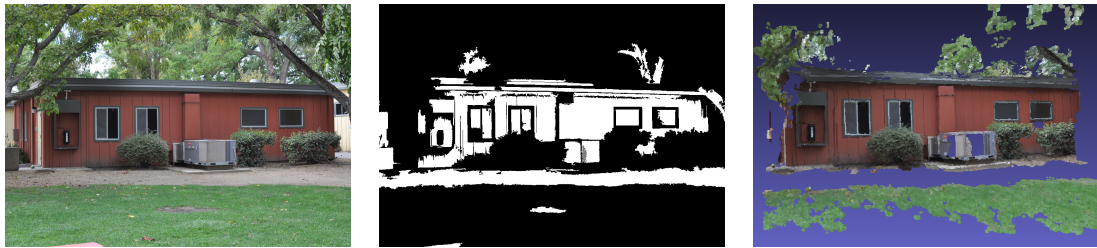
Figure 8: Reconstructed results integrated from our planar- and point-reconstruction methods, rendered by Mesh Lab. One of the reference images ( left ), the masked image ( middle ), the reconstructed scene ( right ).
