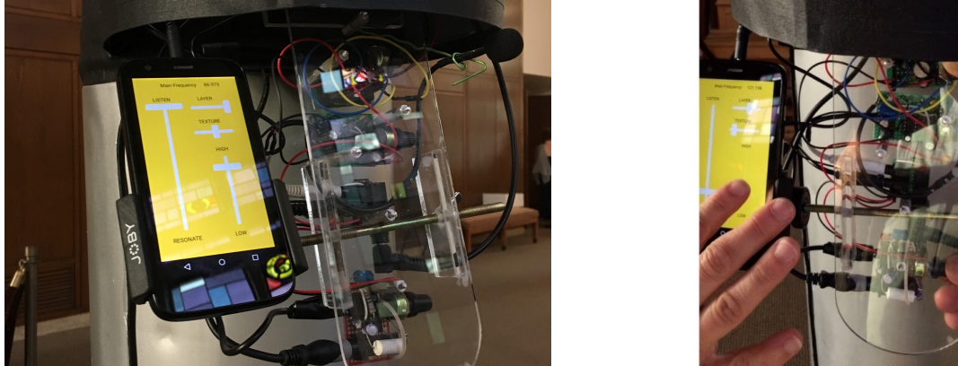
Figure 42. Left: acrylic circuit mounting plate. Right: participants moving sliders and knobs to change the sounds and resonances.
