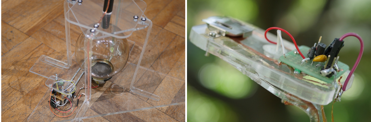
Figure 26. Left: TONE amplifier mounted to acrylic base. Right: TONE preamplifier mounted to an acrylic “leaf.”
