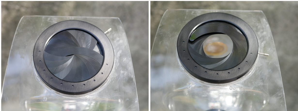
Figure 39. Left: sliding aperture closed. Right: sliding aperture slightly open.
