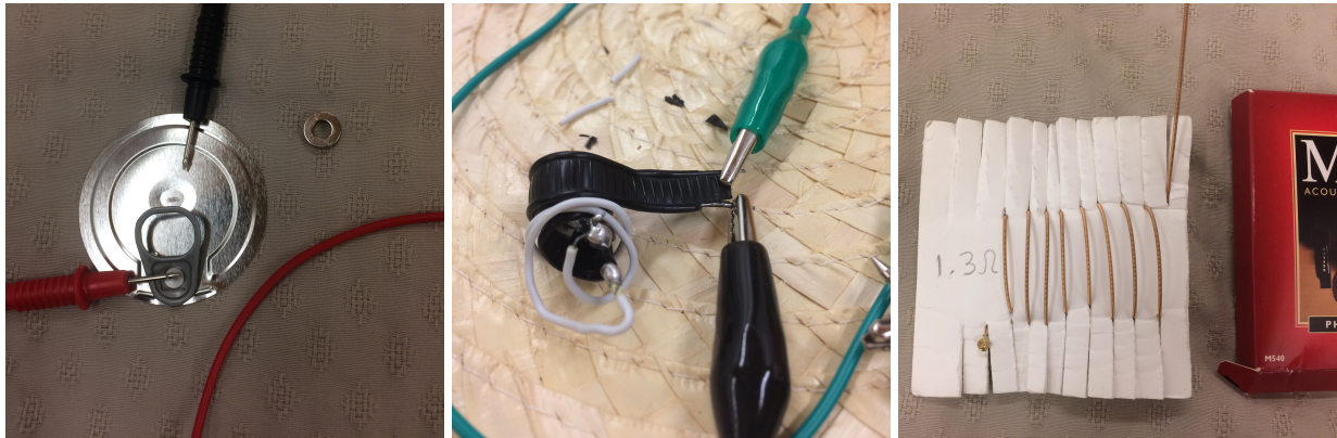
Figure 11. Left: testing an aluminum can lid for electrical continuity. Middle: testing coffee wire coil. Right: guitar string coil ohm reading.
