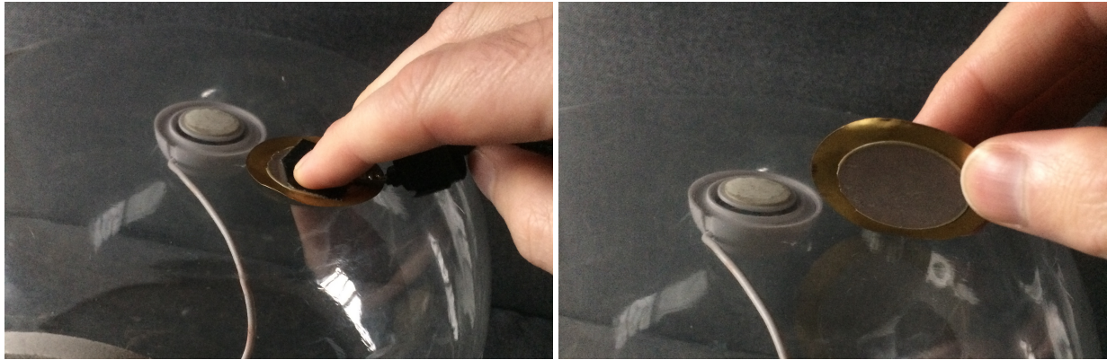
Figure 35. Left: piezo flat on surface. Right: piezo angled on surface.
