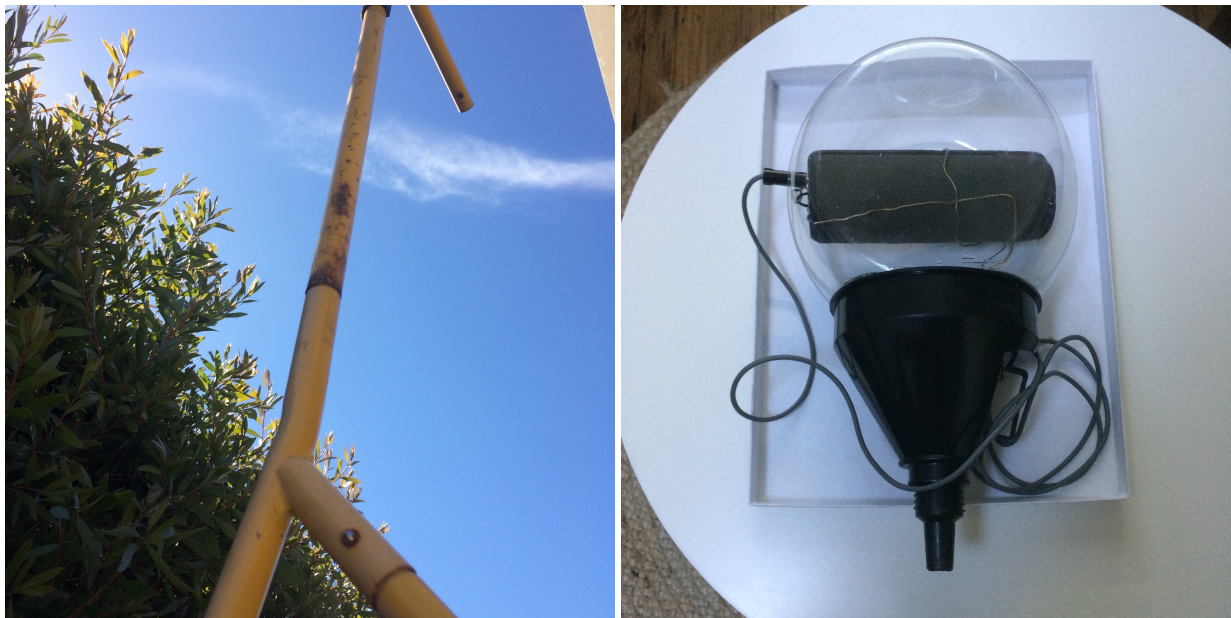
Figure 21. Left: soccer goal frame pipes which snap together. Right: fish bowl hermetically sealed loudspeaker casing.
