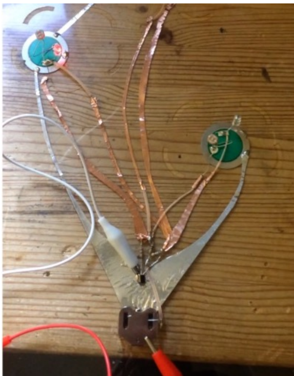
Figure 18. Left: arranging the BLOOM window oscillator digital diagram before building. Right: testing BLOOM circuit with alligator clips to battery.
