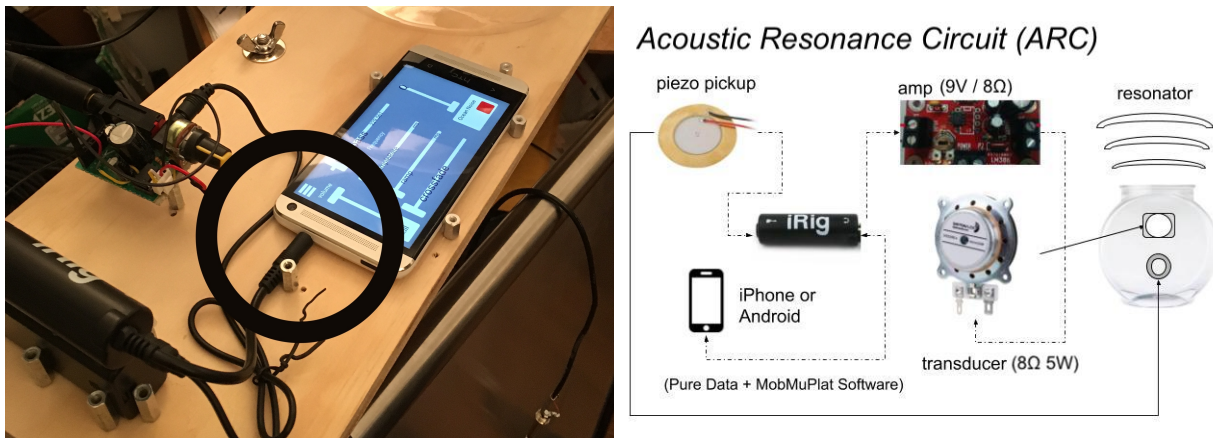
Figure 52. Left: Plug 1/8" TRSM phone jack into smartphone audio jack. Right: Diagram for entire instrument connection scheme.
