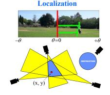
•Pan actuator uncertainty angle prevents accurate triangulation, and defines a detection triangle
