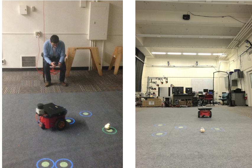
Figure 6.14: The experiment setup. Left: a participant is remotely controlling the Sphero BB-8 to clear the target that he believes will be third in the P3-DX’s sequence. Right: the VICON system (infrared cameras) and the projector.
