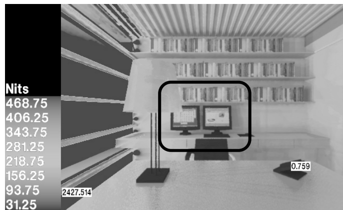
Figure 2. Glare test for a typical office in the e-Lab building using photo-metrically accurate lighting simulation.
