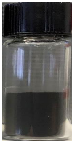
Figure 4-5. Illustration of tape density measurement of 2.5 g LTSO/C in a 4 ml glass vial.
