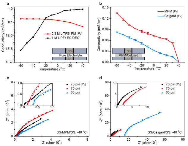
Figure 8: (a) Ionic conductivity of pure electrolyte. (b) Ionic conductivity of LGE with the presence of MPM or Celgard-based membranes as the separator at different temperatures. Nyquist impedance of cells with MPM (c) or Celgard-based (d) membrane as the separator at -40°C and different FM pressures.
