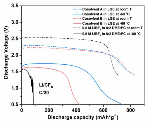
Figure 3: Discharge of Li/CFx using cosolvent A and B in LGE at -60 °C
