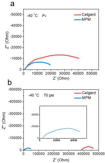
**Figure 10**: Nyquist impedance of  $\text{Li/CF}_x$  mixed with 20% wt UiO-66 using Celgard and MPM at (**a**) vapor pressure and (**b**) 70 psi at -40 °C
