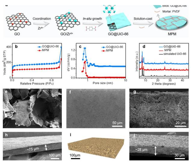
**Figure 7**: (a) Fabrication process of MPMs. N<sub>2</sub> sorption isotherm curves (b) pore size distributions (c), XRD patterns (d) of simulated UiO-66, GO@UiO-66 and MPM. (e) SEM images of GO@UiO-66. Top (f) and cross-sectional (g, h, j) SEM views of two representative MPMs (i)Nano-CT reconstruction of MPM.
