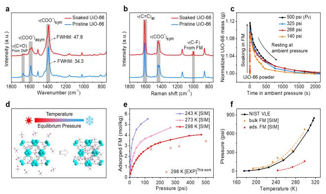
**Figure 6**: FT-IR (a) and Raman spectra (b) of UiO-66 before and after soaking in the FM. c, Mass change test. (d) Schematic of FM in UiO-66 at different conditions. (e) Simulated adsorption isotherms of UiO-66 confined FM. (f) Phase transition comparison between bulk FM and adsorbed FM in UiO-66 systems.
