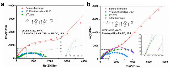
Figure 4: (a) Impedance of ACN-based LGE. (b) Impedance of cosolvent B-based LGE
