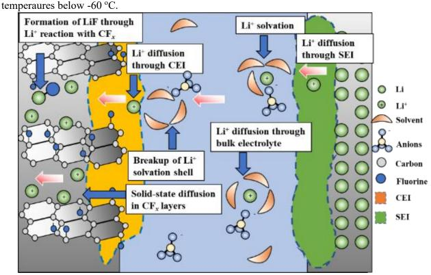
Figure 1: Illustration of discharge process for Li/CF<sub>x</sub> battery
