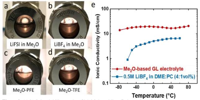
**Figure 2**: (a)(b) Salt solubility results of Me2O-based liquefied gas electrolytes at room temperature (RT). (c)(d) Salt solubility results of well mixed PFE and TFE-based liquefied gas. (e) The conductivity of gas/liquid electrolyte in comparison with liquid electrolyte in temperature range of -80°C to 80°C electrolytes
