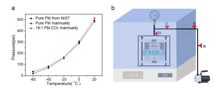
**Figure 11**: (a) Pressure calibration of vapor pressure of FM and the mixture of FM and CO<sub>2</sub> at different temperatures. (b) Schematic description of pressure tuning process.
