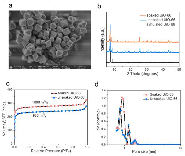
Figure 5: (a) SEM images of UiO-66. XRD patterns (b) N<sub>2</sub> sorption isotherms (c) and pore size distribution profiles (d) of UiO-66 before and after soaked in liquified FM
